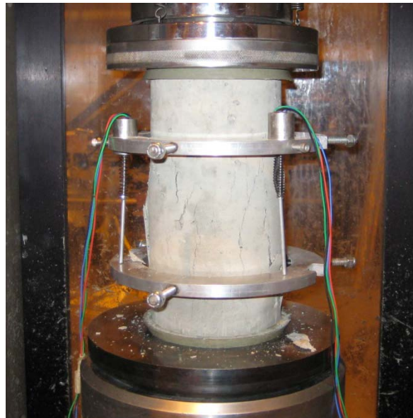
Figure B-5: Cylinder test using a yoke to determine the stress-strain response of the concrete. Two LVDTs are visible and the third is hidden behind the cylinder.
