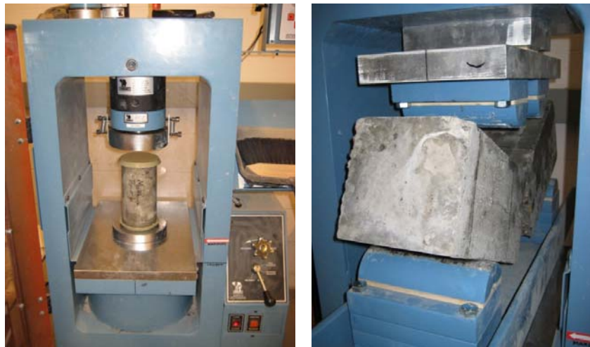
Figure 3-9: Quality control testing of a cylinder (left) and a modulus of rupture test.
