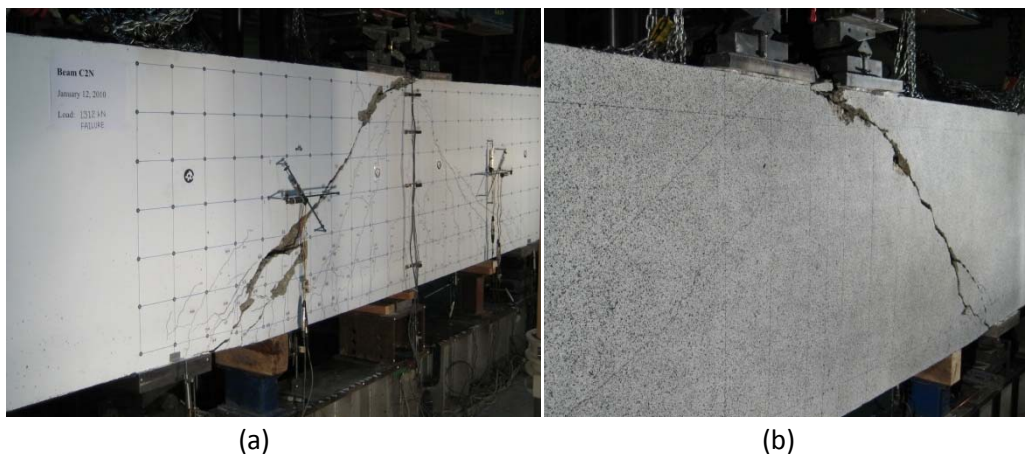
Figure C-147: Failure surface in shear span A from the front (a) and from the back (b) side of specimen C2N.
