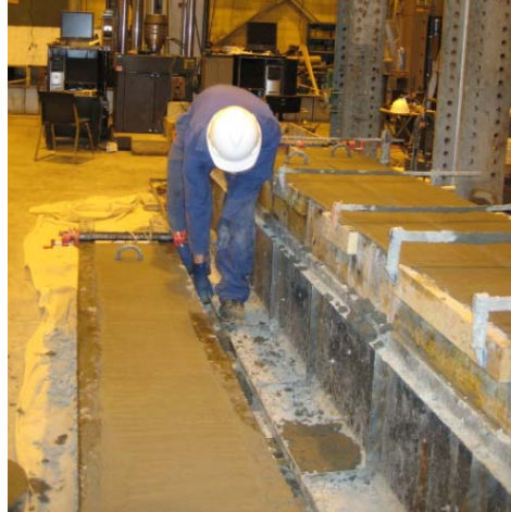
Figure 3-7: Finishing a set of specimens.
