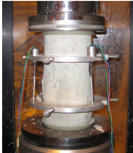
Figure 3-10: Cylinder test with a strain yoke to determine the stress-strain response.
