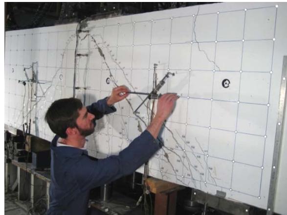
Figure C-132: Specimen C1N after failure occurred in shear span B (center of picture).
