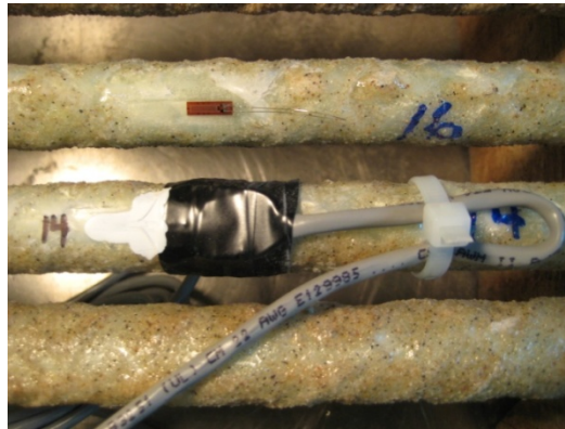
Figure C-3: Instrumentation of the GFRP bars with strain gauges. Middle bar shows a strain gauge with wires attached and covered with M-coat D protective coating. The silicon protective coating has not been added yet.
