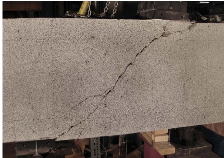
Figure C-94: Back side of specimen B4N showing the failure surface in shear span B.
