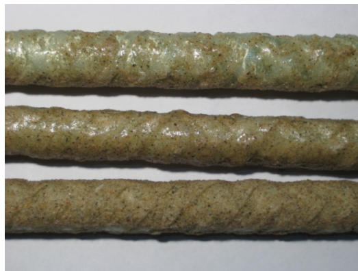
Figure 3-8: GFRP bars, No. 8 at the top and two No. 7.
