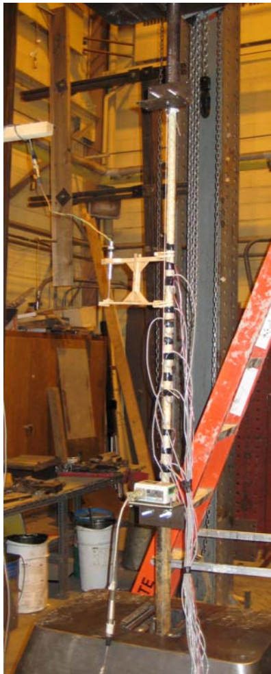
Figure A-5: Typical tension test setup with strain gauges, LVDT, and cable potentiometer.
