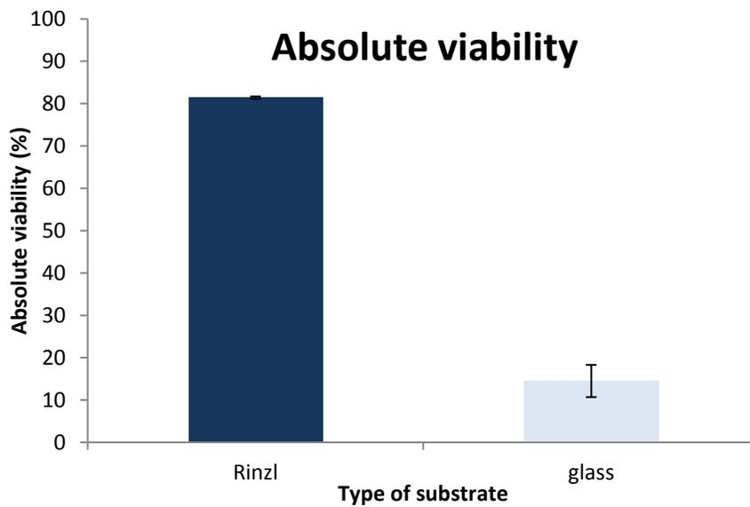
Figure 4.23: Comparison of the maximum absolute viability for HUVECs after plunge- thaw in the presence of 5% DMSO and 6% HES on Rinzl and glass coverslips
