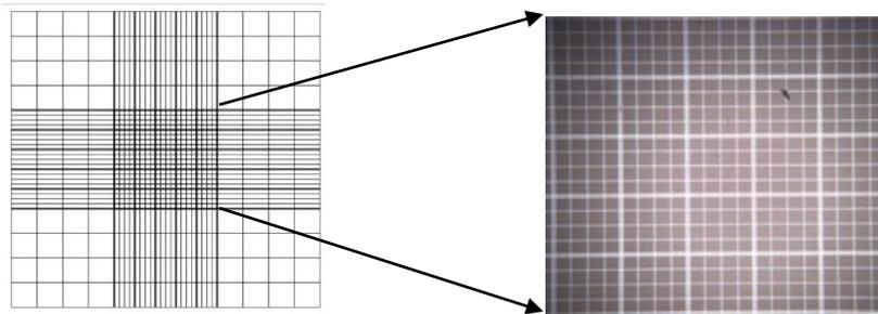
Figure 2.2: Hemacytometer image taken by bright field microscopy (capture resolution: 1280×1024)
