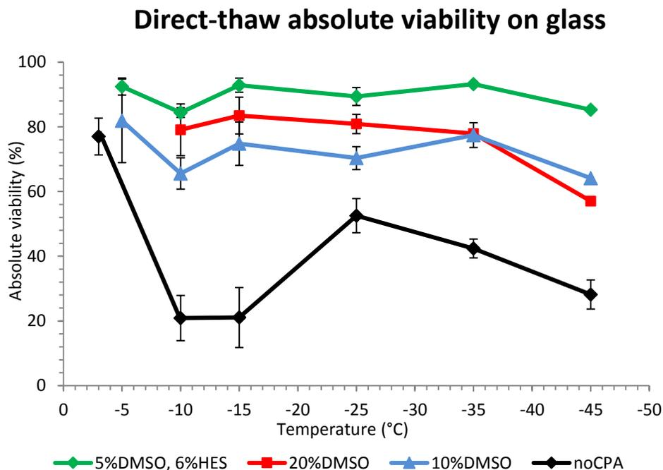
Figure 4.12: Comparison of absolute viability of monolayers on glass coverslips after direct-thaw in the absence or presence of cryoprotectants. Results are the average of three independent experiments. Data are presented as mean  $\pm$  standard error of the mean (SEM).
