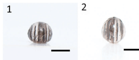
Fig. 4 Photographs of the resulting particles polymerized with a magnet above and below the droplet in the attractive regime. The bottom distance is fixed as 2 cm and both particles are synthesized at center (place I) (5, 5). Top distance for (1) is 5 cm and for (2) is 3.5 cm. All scale bars in the pictures are 1 mm.
