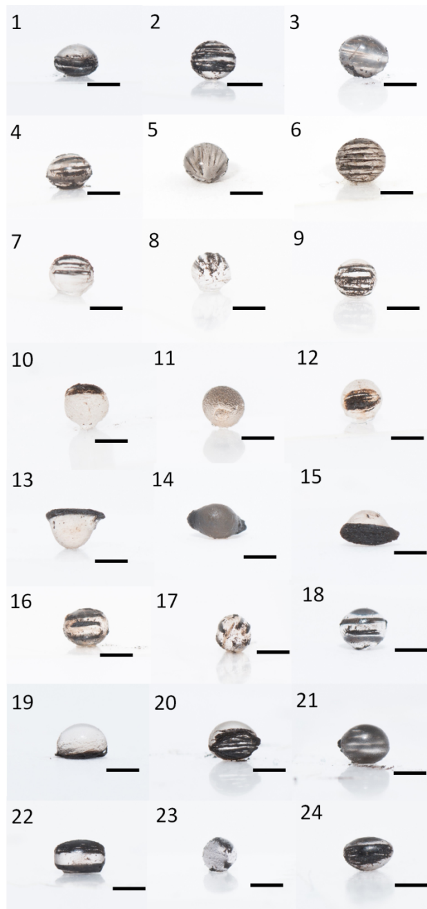
Figure S5. Photographs of the resulting particles polymerized with a magnet above and below the droplet in the repulsive regime. For the photographs in (4-9, 16-18, 22-24) the left panel is a side view of the major axis, the middle panel is side view of the minor axis, and the right panel is a bottom view. Otherwise, all photographs on the left are side views, middle are bottom views, and right are top views. (1-3) The distance between the top magnet and Petri dish is 5 cm, and the distance between bottom magnet and the Petri dish is 2 cm, position (1,1) on the Teflon. (4-6) The distance between top magnet and Petri
