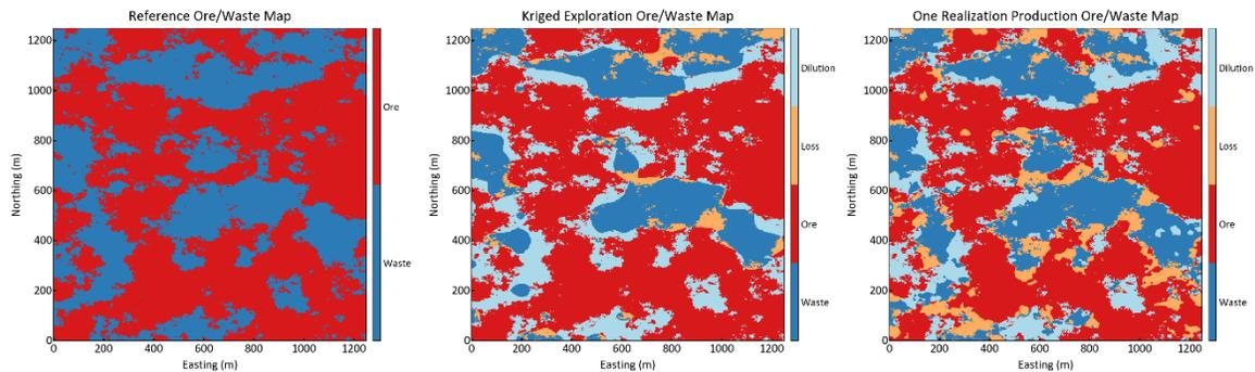
Figure 2.10 – Ore and waste maps calculated on the reference model (left), exploration data kriged estimates (center) and one realization of production data estimates (right).
