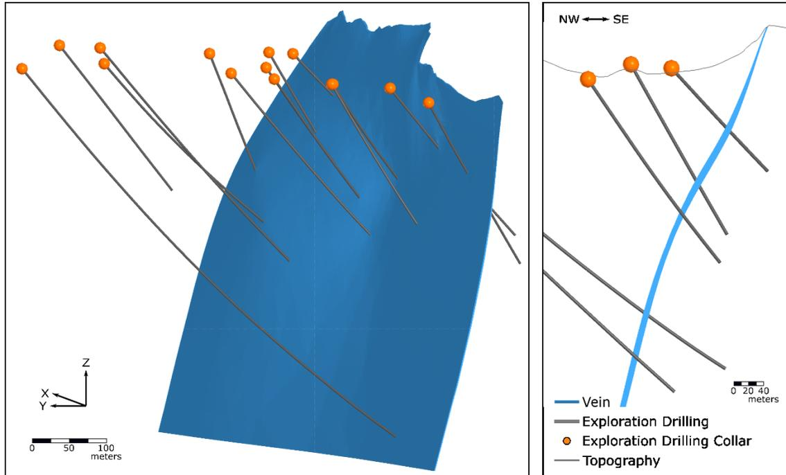
Figure 5.6 – Perspective (left) and section (right) views of the vein and exploration data.
