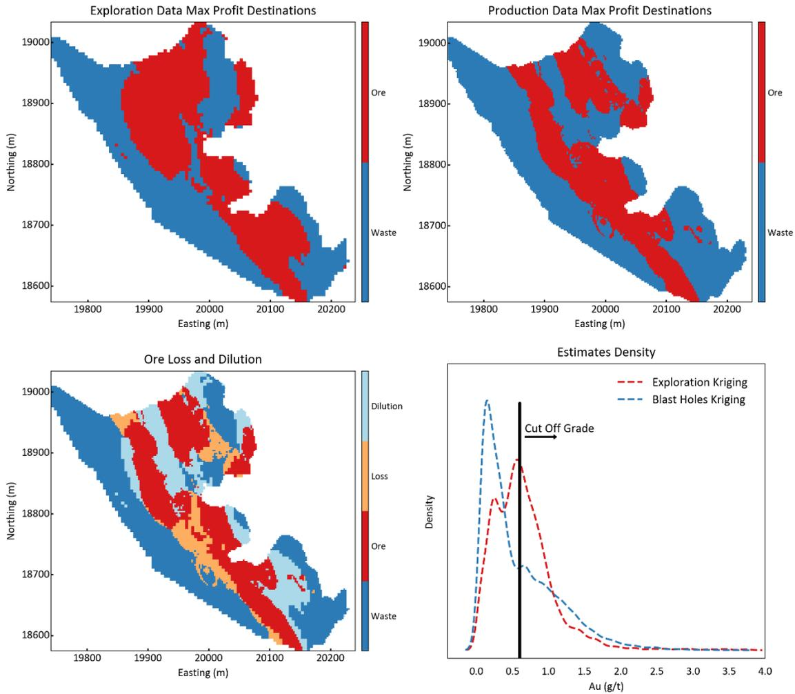
Figure 2.4 – Ore and waste maps on the exploration (top left) and production data (top right) estimates, ore loss and dilution map (bottom left) and estimates histograms (bottom right).
