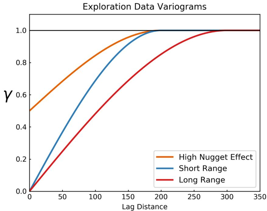
Figure 4.17 – Exploration data variogram models used in the workflow.
