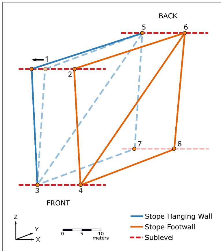
Figure 5.5 – A schematic perspective view of a stope optimization where the stope orientation is consistent with the original coordinates system. The key eight points that define the stope vary along the X axis only.
