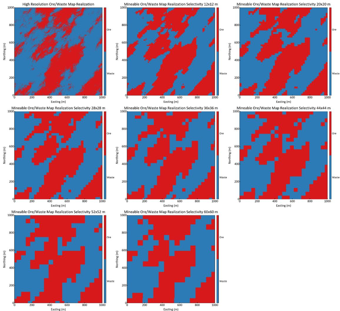
Figure 4.14 – Ore and waste location maps for one realization for increasing minimum mineable unit size.
