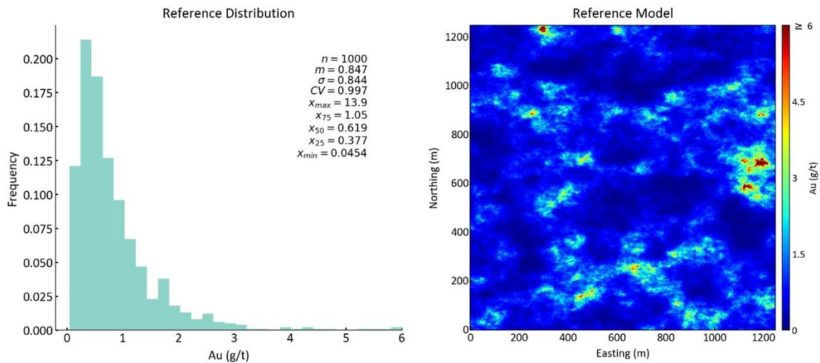
Figure 2.5 – Reference grade distribution (left) and reference gold model (right).
