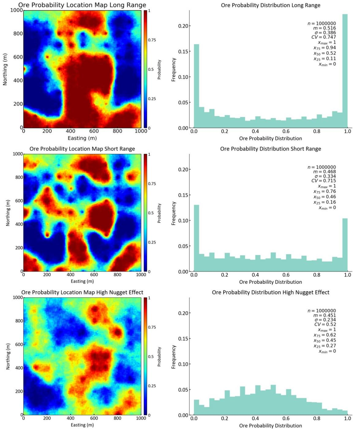
Figure 4.18 – Ore probabilities locations maps and histograms for three different exploration data variogram models: long range variogram (top), short range variogram (center) and high nugget effect variogram (bottom). Note that the Y axis scale is the same for all histograms of ore probabilities to showcase their differences.
