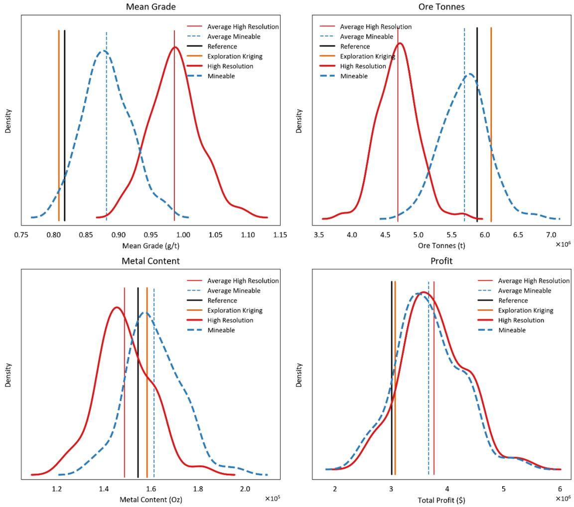
Figure 4.7 – Distributions of resources calculated on the reference model (black), the kriged estimates of exploration data (orange), the high resolution simulated realizations (red) and going through the proposed workflow (blue).
