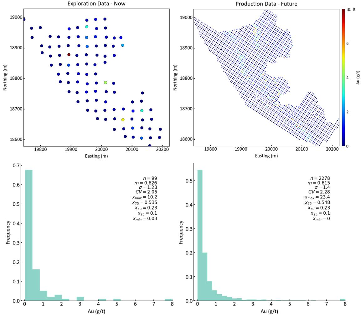
Figure 2.2 – Sampled exploration data (top left) and bench production dataset (top right) and their gold grades histograms (bottom).
