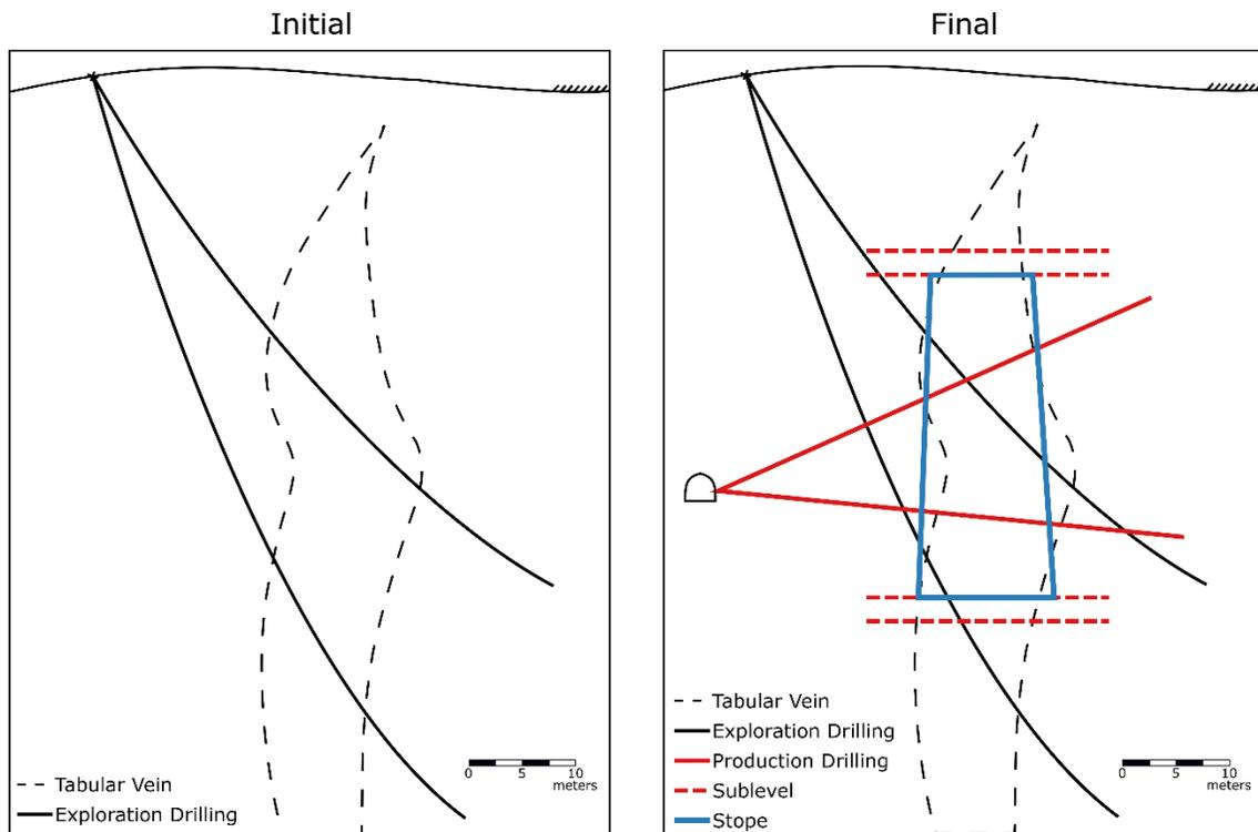
Figure 5.1 – Schematic cross section views illustrating typical initial (left) and final (right) data configurations of a subvertical tabular vein deposit.
