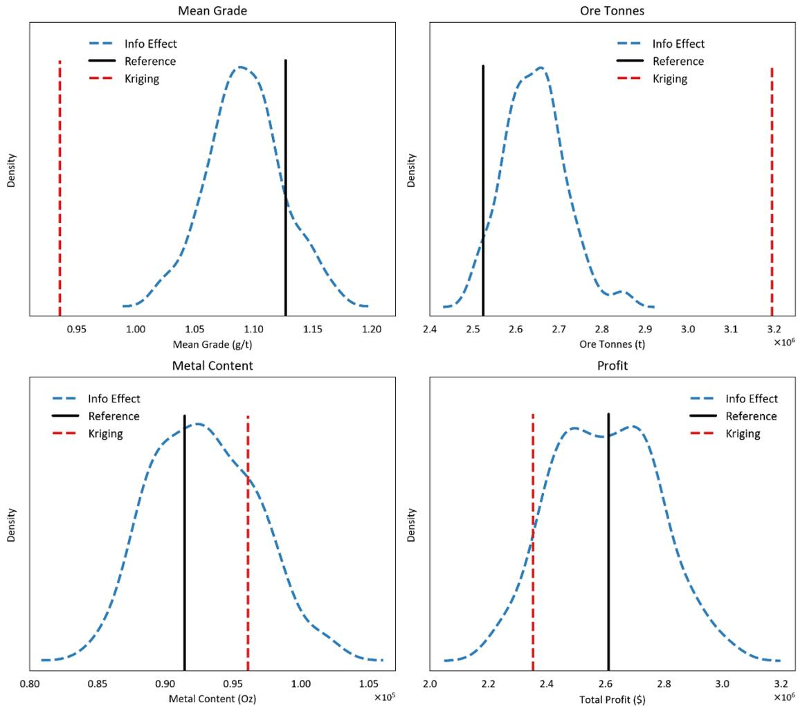
Figure 2.11 – Mineral resources for the entire bench: mean grade (top left), tonnes of ore (top right), metal content (bottom left) and total profit (bottom right).
