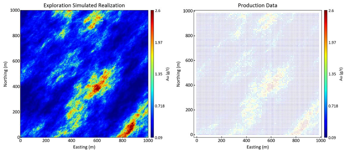
Figure 4.4 – Simulated realization with exploration drill holes (left) and blast holes sampled from it (right).
