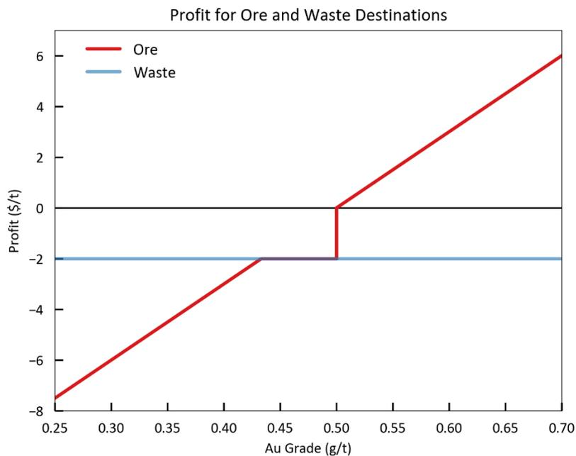
Figure 3.3 – Expected profits for ore and waste grid cells.
