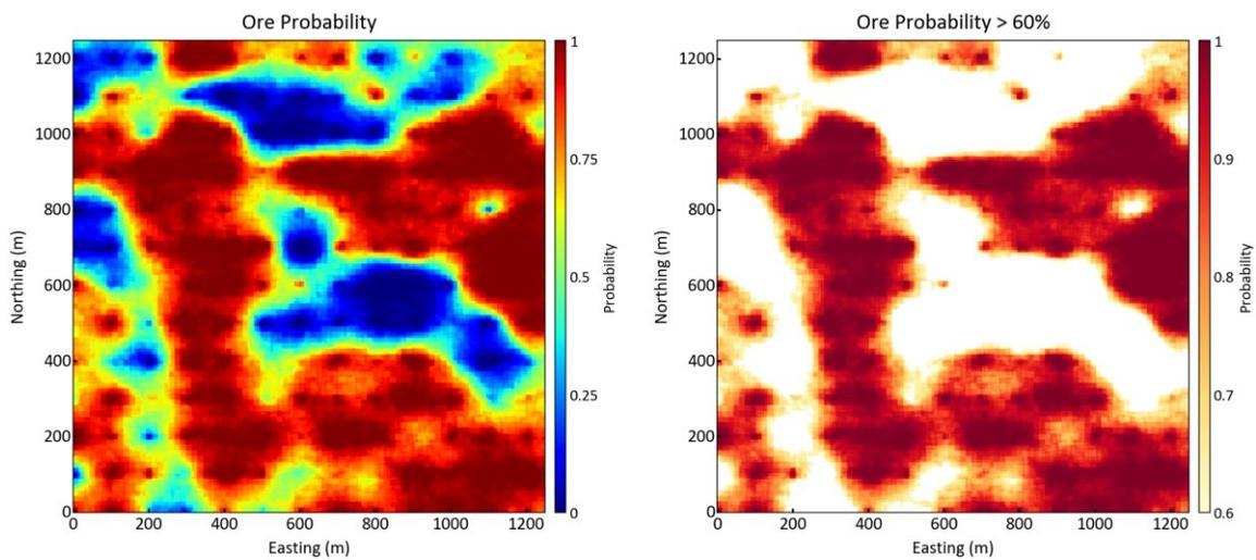
Figure 3.6 – Ore probability map (left) and the grid cells where the ore probability is greater than 60% (right).
