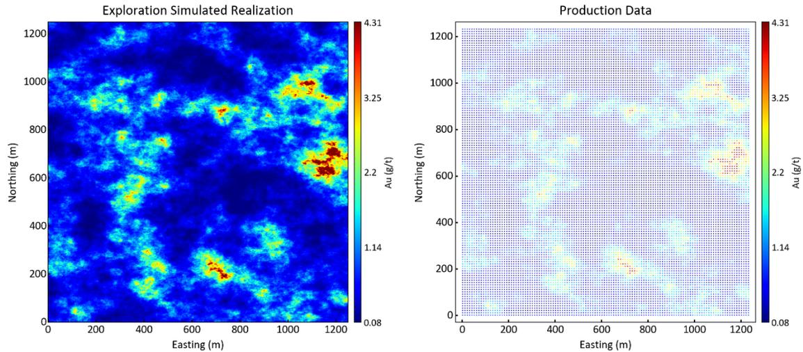
Figure 2.7 – One exploration simulated realization (left) and the sampled production dataset (right).
