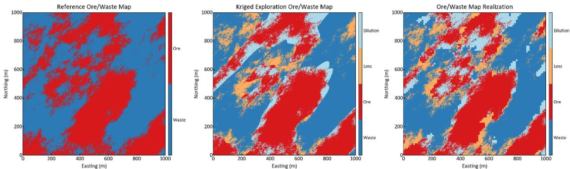
Figure 4.8 – Ore, waste, ore loss and dilution location maps.
