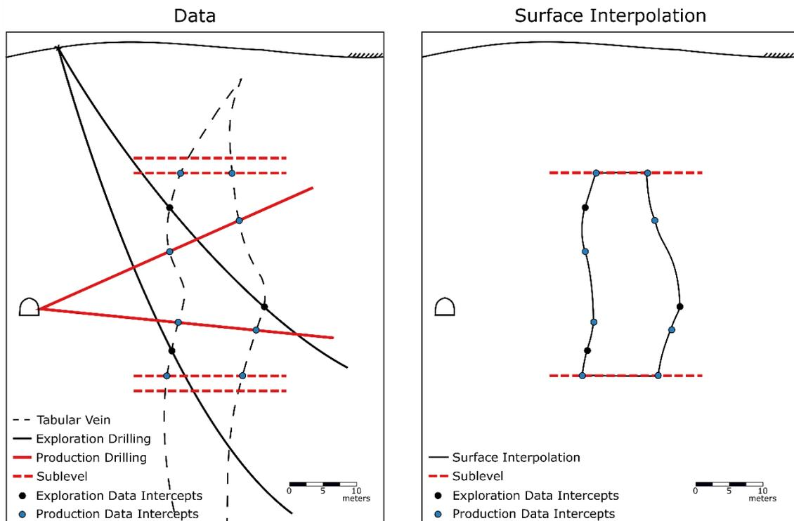
Figure 5.2 – Schematic cross section views of a mineralized vein illustrating the data intercepts with a vein surface realization (left) and the interpolated vein surface (right).
