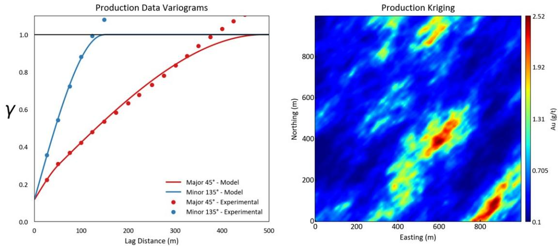
Figure 4.5 - Experimental variograms calculated with production data and fitted variogram model (left) and their estimates (right).
