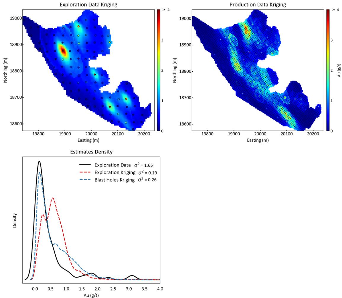
Figure 2.3 – Estimated exploration (top left) and blast holes (top right) datasets and histograms of the estimates (bottom).
