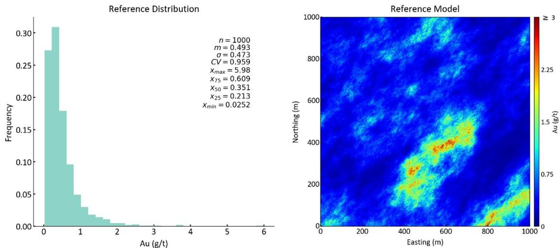
Figure 4.2 – Reference grade distribution (left) and reference gold gridded model (right).
