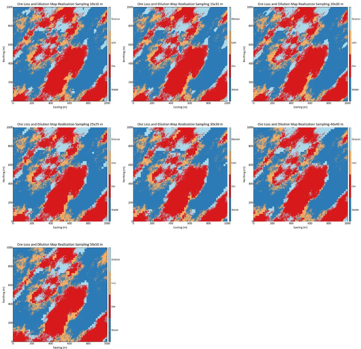
Figure 4.11 – Ore, waste, ore loss and dilution location maps of one realization of the workflow for increasing grade control data spacing.
