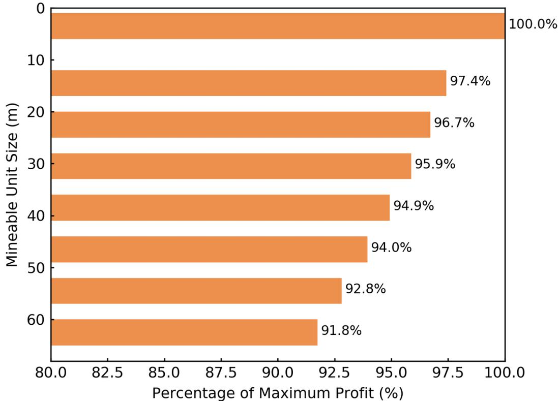
Figure 4.16 – Percentages of maximum profit achievable at the time of mining and the minimum mineable unit sizes.
