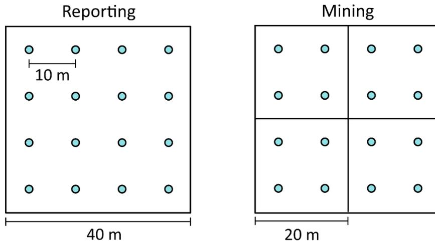
Figure 3.1 – Contrasting SMU sizes used for resources reporting (left) and operational grade control model (right). The anticipated final grade control data spacing is presented in blue.
