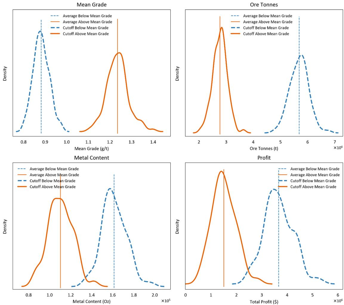
Figure 4.21 – Distributions of resources calculated on the base case scenario (cutoff below mean grade of the bench – blue) and for the cutoff above the mean grade (orange).
