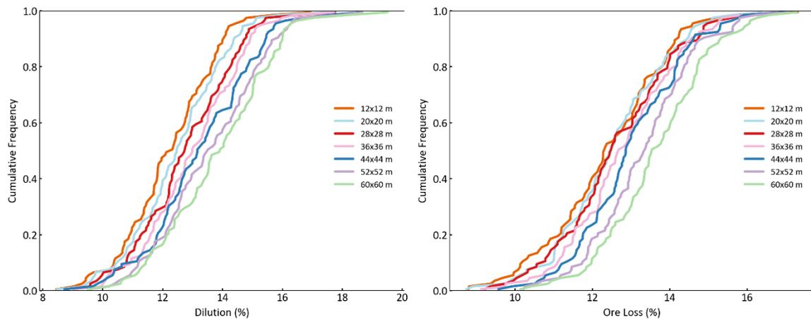
Figure 4.15 – Percentages of dilution and lost ore for varying mineable unit sizes.
