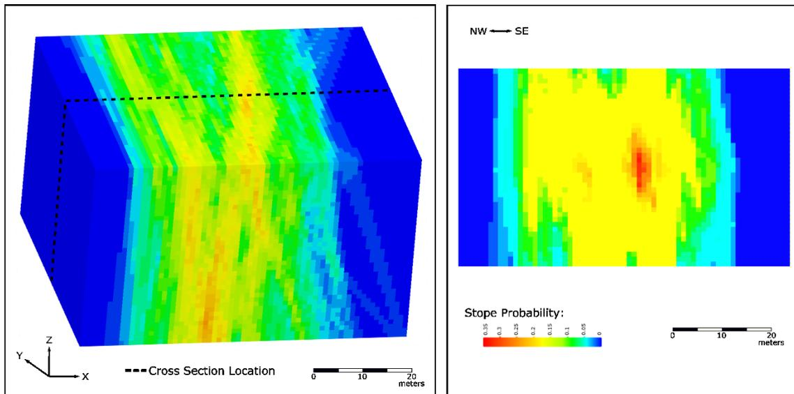
Figure 5.13 – Perspective (left) and cross section (right) views of the probability of a grid cell to be inside the optimized stopes for a hundred realizations.
