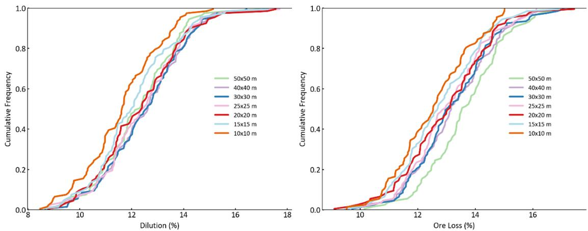
Figure 4.12 – Percentages of dilution and lost ore for varying production data spacing.
