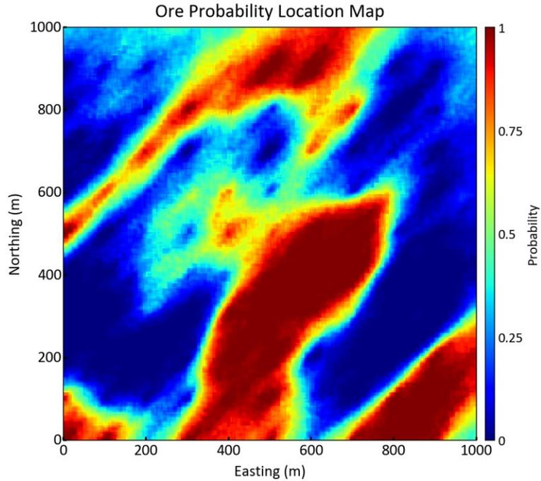
Figure 4.9 – Ore probability map of simulated model going through the proposed workflow.
