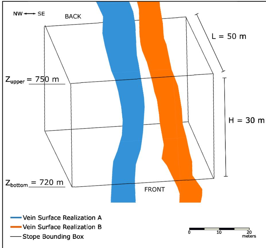
Figure 5.7 – Cross section views of two surface realizations and stope bounding box in perspective.
