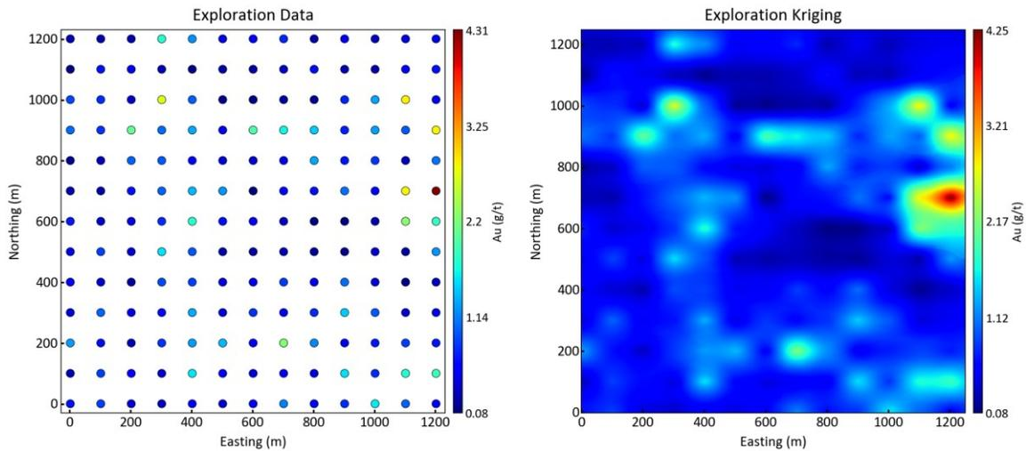
Figure 2.6 – Exploration data sampled from reference model (left) and estimates (right).
