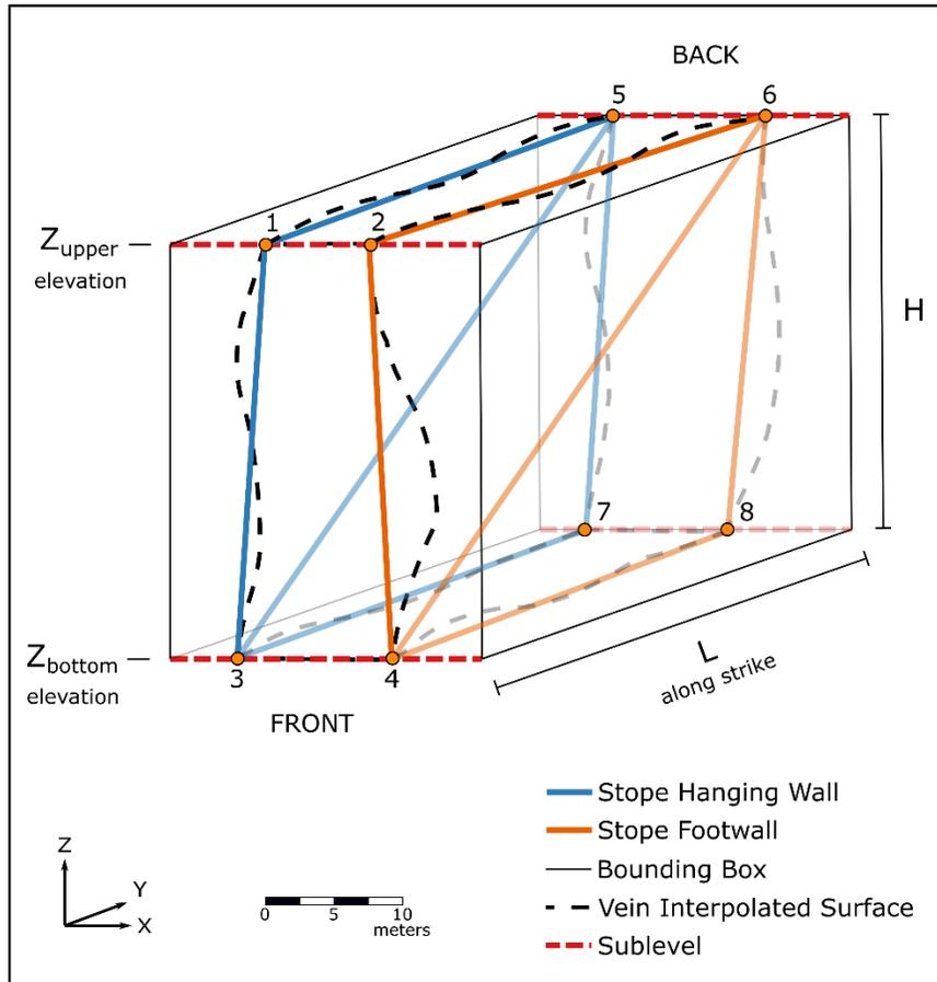
Figure 5.3 – A schematic perspective view of a stope in a steeply dipping mineralized vein.
