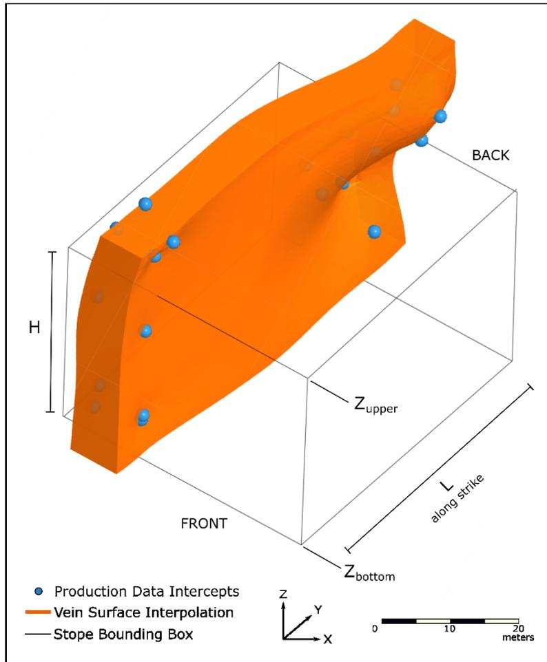
Figure 5.8 – Perspective view of production data intercepts and vein surface interpolation.
