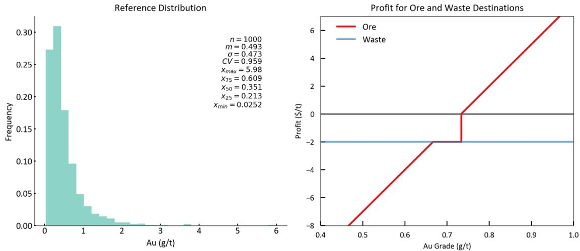
Figure 4.20 – Reference grade distribution (left) and expected profits for ore and waste.
