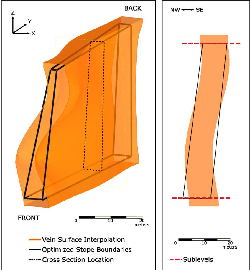
Figure 5.10 – Perspective view (left) and cross section (right) of optimized stope boundaries for one reinterpolated vein surface.
