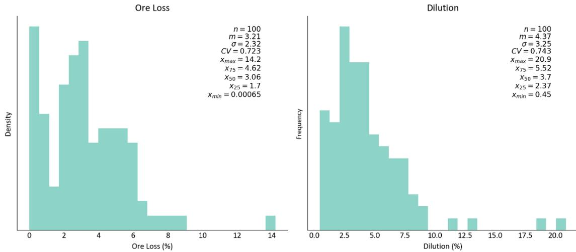
Figure 5.12 – Ore loss (left) and dilution (right) relative to the optimized stopes volume for each realization.
