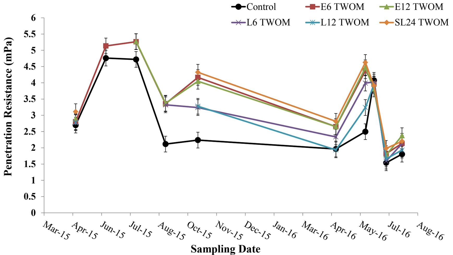
**Figure 2-3.** Penetration resistance (PR) of Control and traffic without mats (TWOM) treatments on loam soils.
