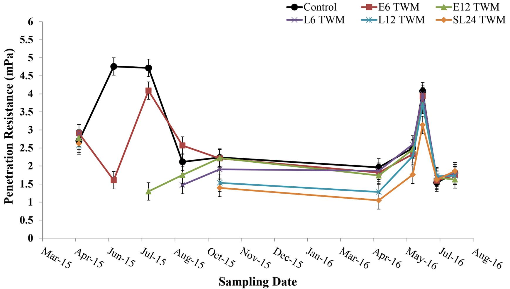
**Figure 2–5.** Penetration resistance (PR) of Control and traffic with mats (TWM) treatments on loam soils.
