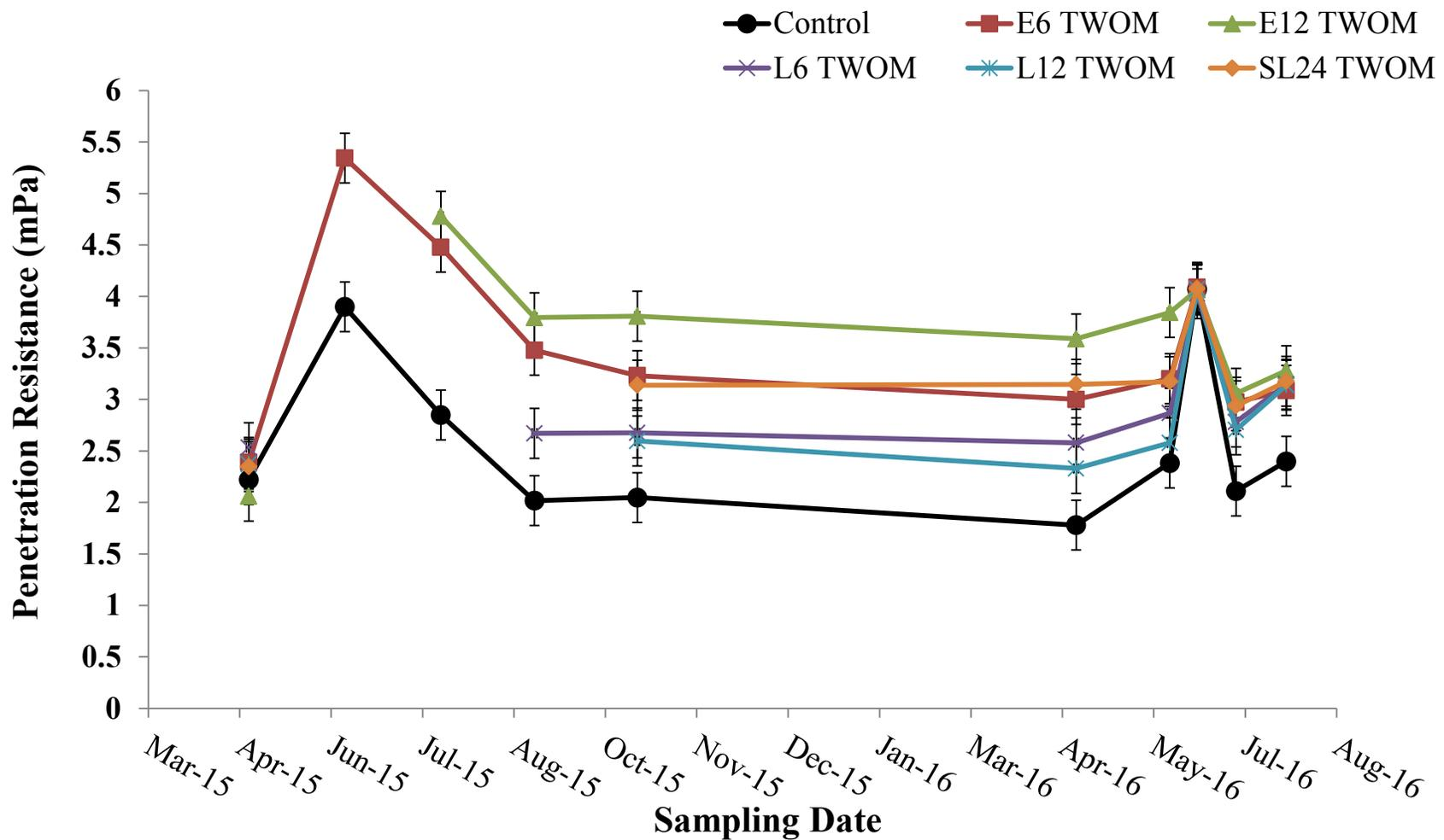
**Figure 2–4.** Penetration resistance (PR) of Control and traffic without mats (TWOM) treatments on loamy-sand soils.
