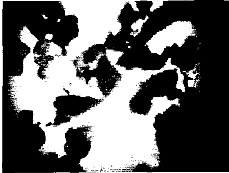
Figure 49 Stereomicroscopic image of roasted (1000°C 30') SB40 heavy product under transmitted light (Magnification = 60)
