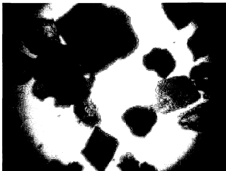
Figure 46 Stereomicroscopic image of roasted (900°C 30') SB40 heavy product under transmitted light (Magnification = 60)
