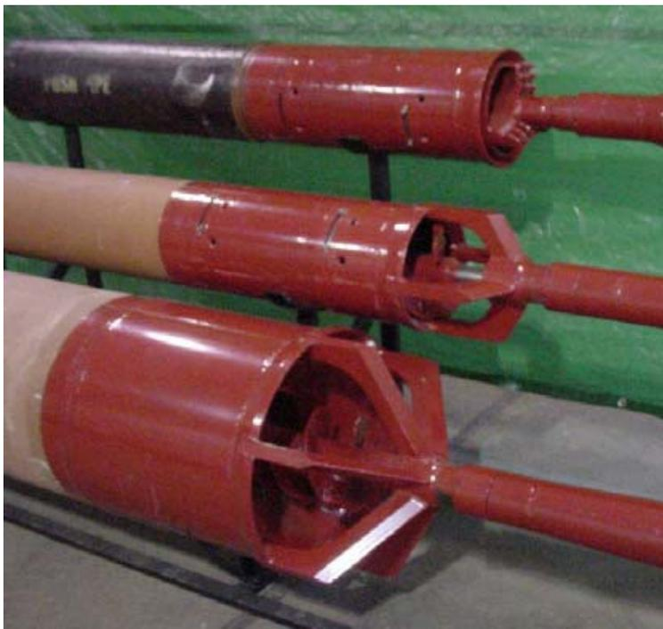
**Figure 2.7 Reaming heads for GBM (Boschert 2007)**
