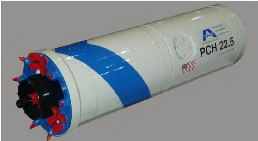
**Figure 2.10 Powered cutter head from Akkaerman (Gottipati 2011)**
