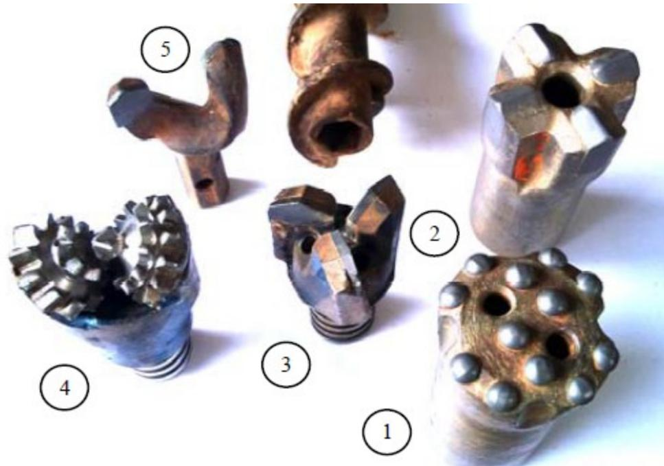
**Figure 2.19 Drilling bits used: 1: button bit, 2: cross-type bit, 3: drag bit, 4: bicone roller bit 5: continuous flight auger (Laudanski et al. 2014)**
