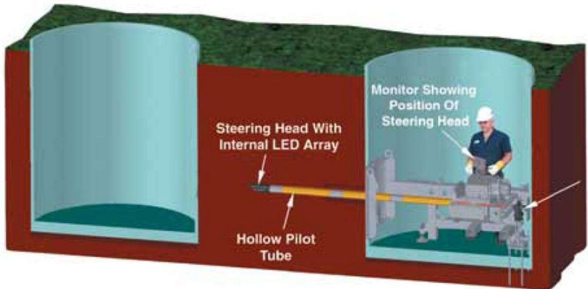
**Figure 2.2 Precise installation of pilot tubes (Akkerman 2013)**
