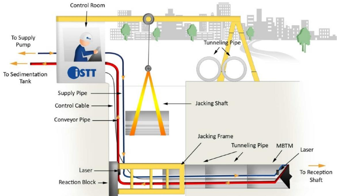
Figure 2.15 Pipe installation using microtunnelling (ISTT 2015).
