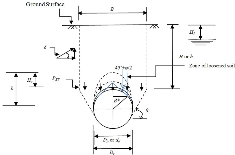
**Figure 4.1 Typical cross section of pipe during pipe jacking**
