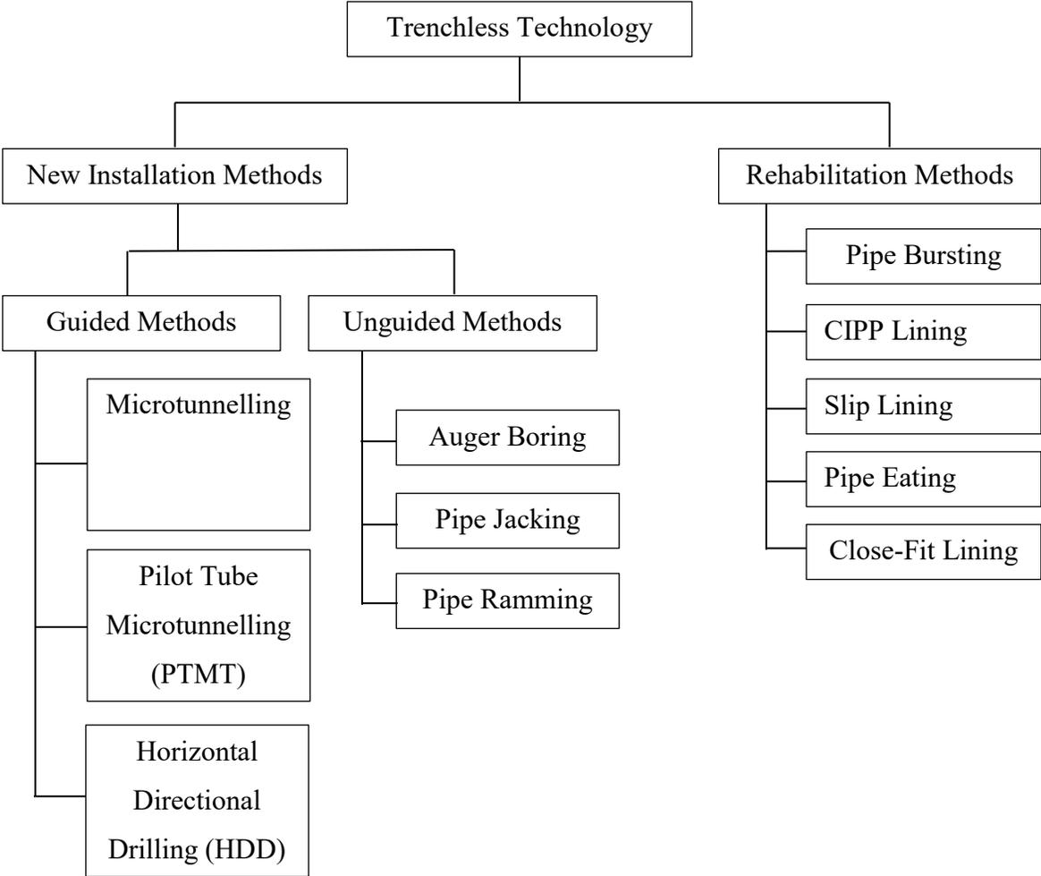
**Figure 2.1 Family of trenchless technologies adapted from ISTT 2011 (Gottipati 2011)**
