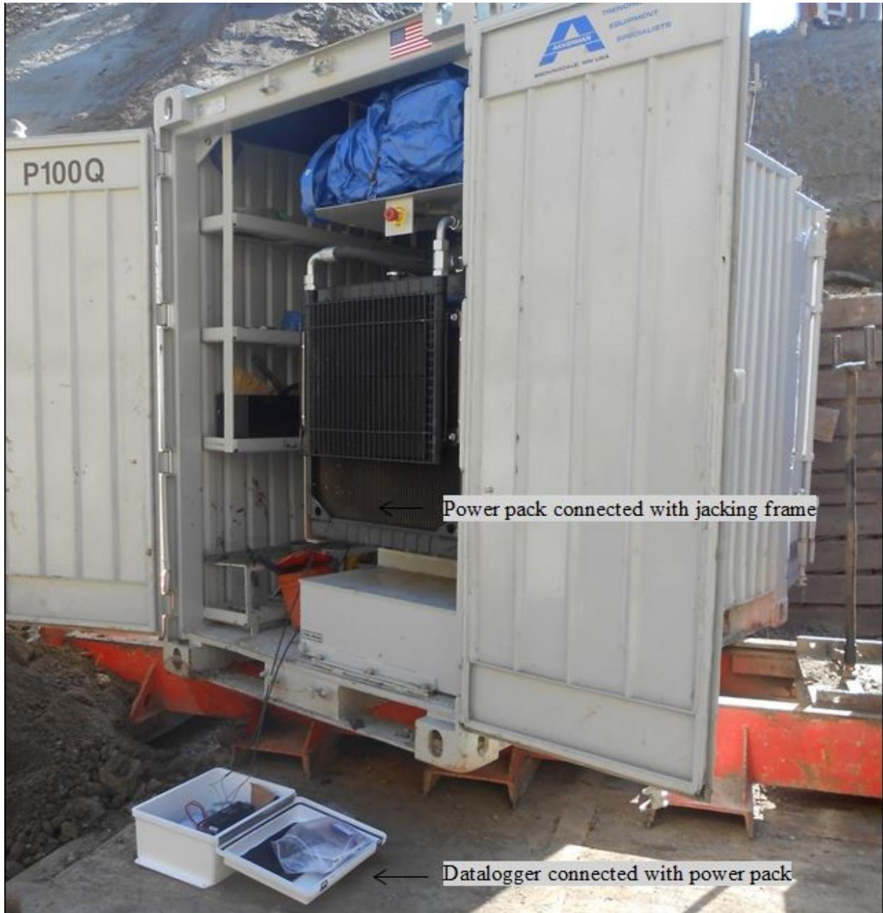
**Figure 3.6 Continuous measurement of data using Datalogger**
