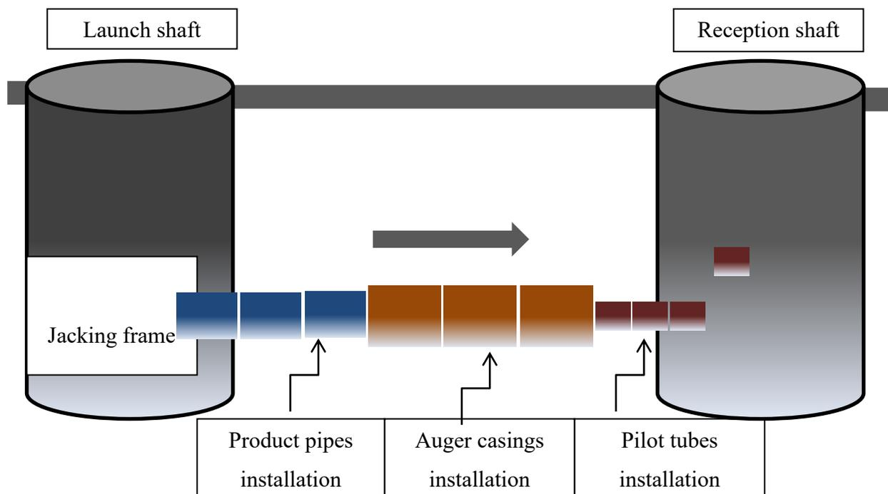
Figure 3.1 Three-step installation procedure of GBM
