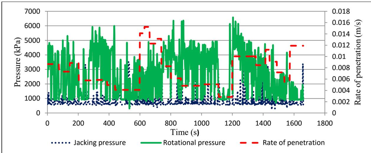
**Figure 3.7 Recorded jacking pressure, rotational pressure, and rate of penetration**
