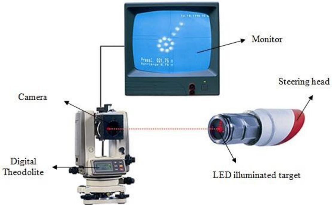
**Figure 2.4** Guidance system for GBM adapted from ISTT (2011) (Gottipati 2011)
