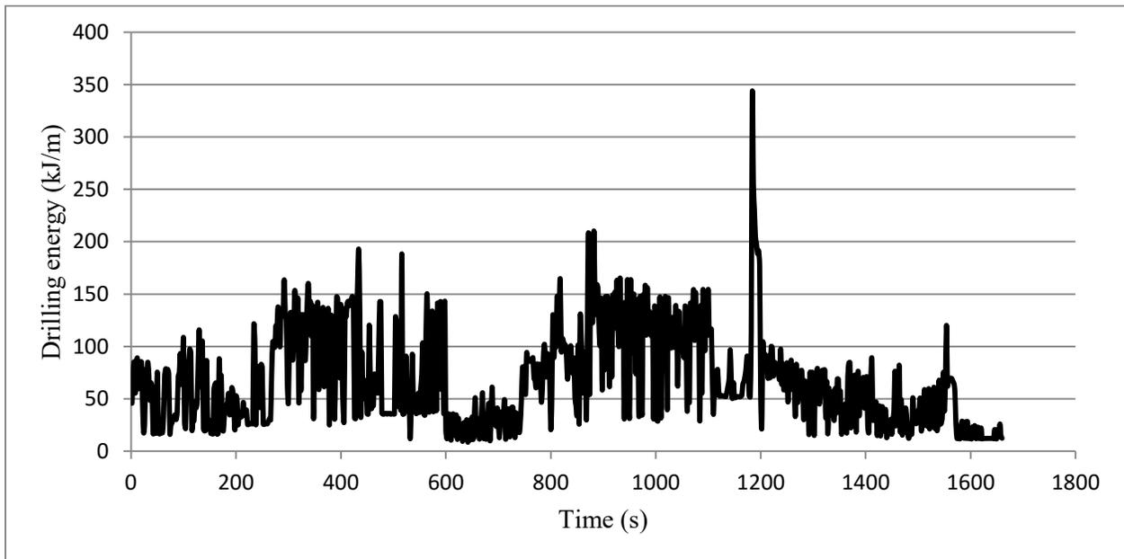
**Figure 3.12 Energy required for drilling defined by Pfister (1985) vs time**
