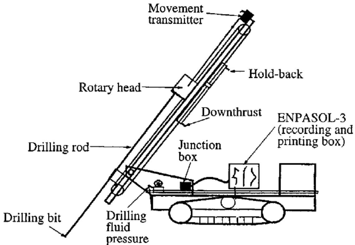
Figure 2.18 Typical instrumented rotary drilling rig (Gui et al. 2002)
