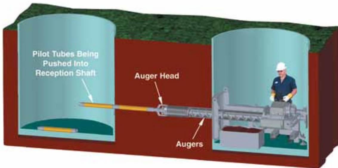
**Figure 2.5 Auger casings' installation along the pilot tube path (Akkerman 2013)**
