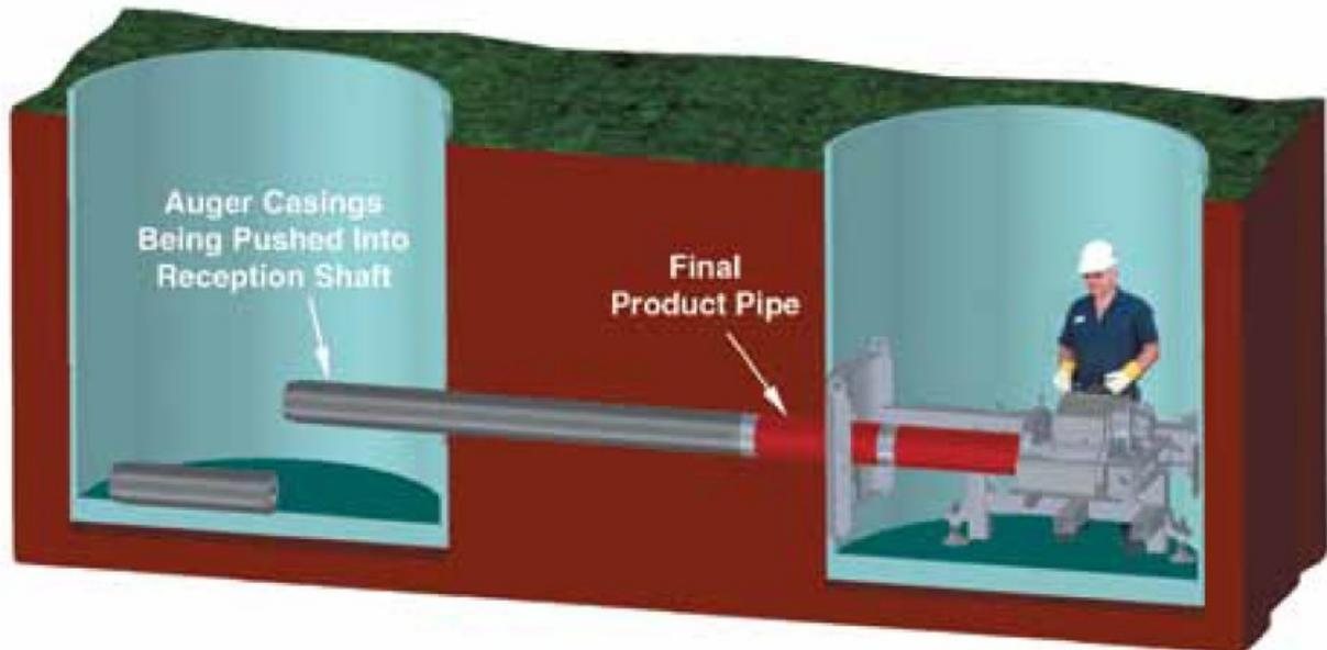
**Figure 2.8 Final product pipes installation (Akkerman 2013)**
