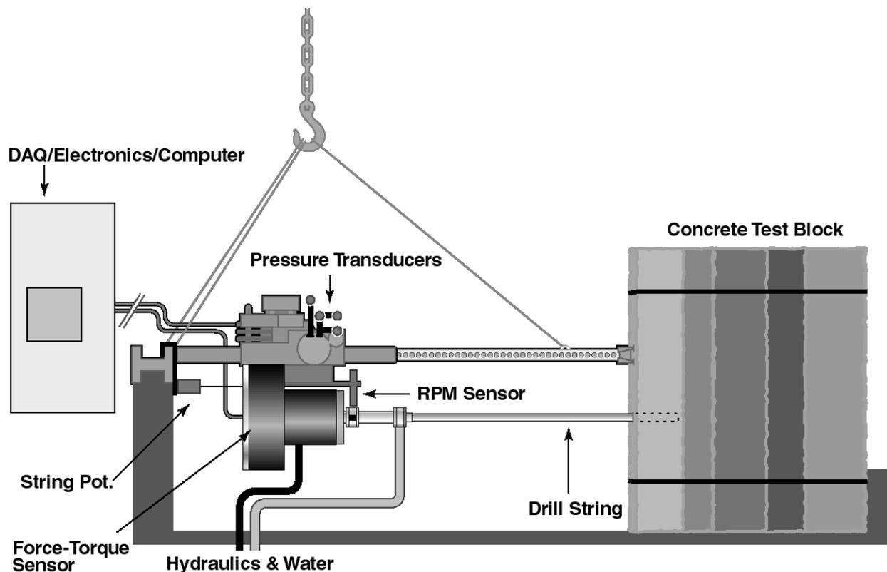
**Figure 2.17 Laboratory drill apparatus and set-up (LaBelle 2001)**
