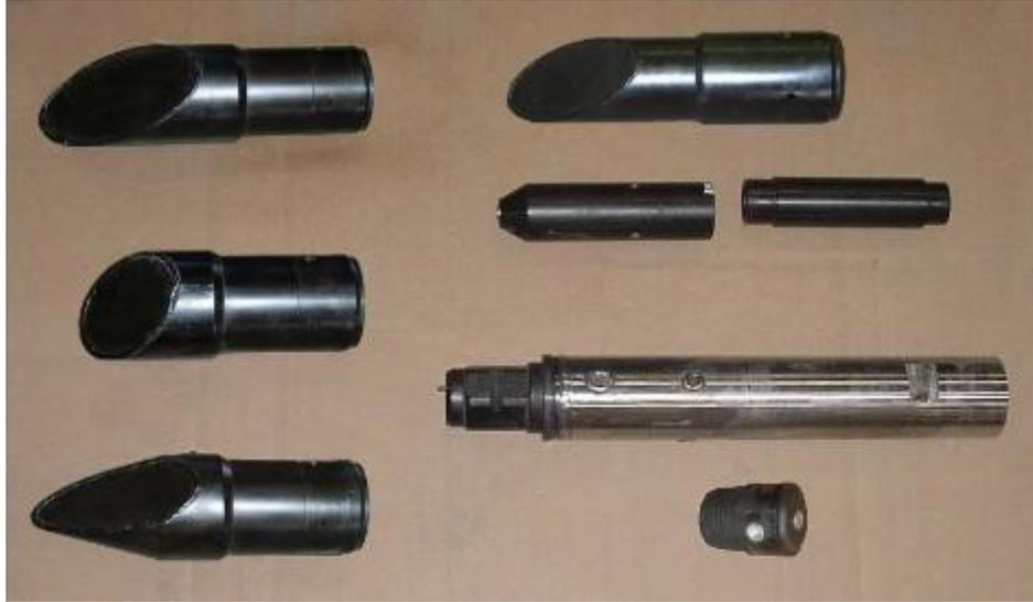
**Figure 2.3** Various types of steering heads and supporting equipment adapted from Akkerman (2010) (Gottipati 2011)
