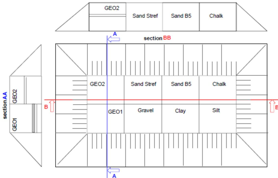
**Figure 2.20 Schematic plan of the embankment built by Rouen Experimental Station (Laudanski et al. 2014)**
