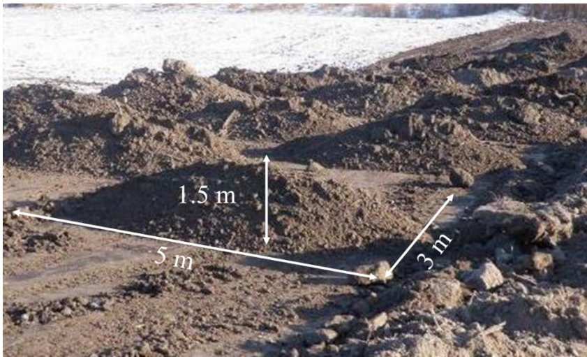
Figure 3.6-2: Material layering scheme of hills and hill dimensions following placement on the research slope.
