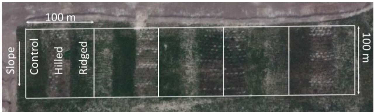
Figure 2.5-1 (a) Aerial view of the overburden dump with the south and east research slopes outlined in red. (b) Aerial view showing one of the two research slopes and the five replication blocks with microtopographic treatments.
