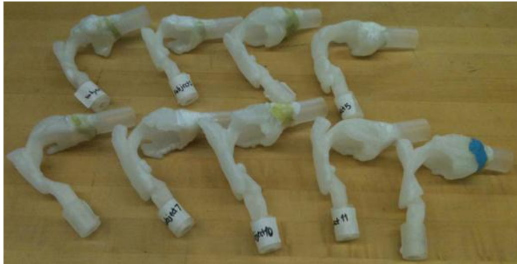
Figure 4.2 Nine oral airway replicas of children 6-14 years old. The replicas are arranged in an ascending order based on their numerical label from left to right on each row.
