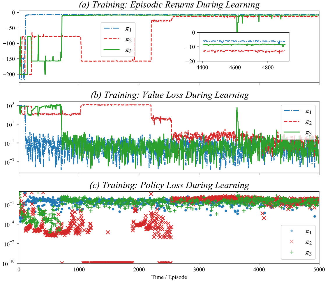
Figure 5.6: Performances of three policies during training. (a) Episodic return (equation (5.1)) is a common performance metric. In the ideal case, it should converge to zero, however, the maximum value is -5 in this problem due to the initial position of the cropping box. As shown in the figure, the noise corrupts \pi_2 initially and delays the learning of a good policy significantly. It also has a lower asymptotic return compared to the other policies. On the other hand, \pi_3 results in a closer asymptotic performance to \pi_1 due to the PF. (b) The A3C agent tries to minimize the TD-error by optimizing the critic loss shown in equation (5.8). The figure shows that \pi_1 and \pi_3 can minimize the value loss quickly, however, the noise in \pi_2 causes huge value losses, especially between episodes 1000 and 2000. (c) Since the policy is also optimized by using the TD-error, its loss should be stable to avoid numerical issues. \pi_1 and \pi_3 demonstrate similar performances in terms of the policy loss as expected. However, the excessive noise causes \pi_2 to become unstable between episodes 1000 and 3000.
