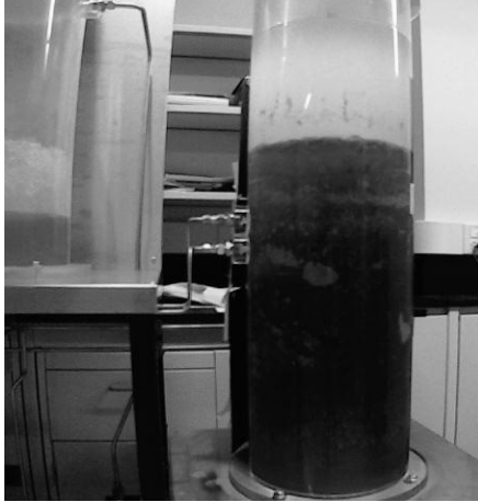
Figure 6.1: Experimental, pilot-scale PSV setup. The black liquid (a water mixture) represents the middlings, the white liquid (oil) mimics the froth layer in the industrial setup.
