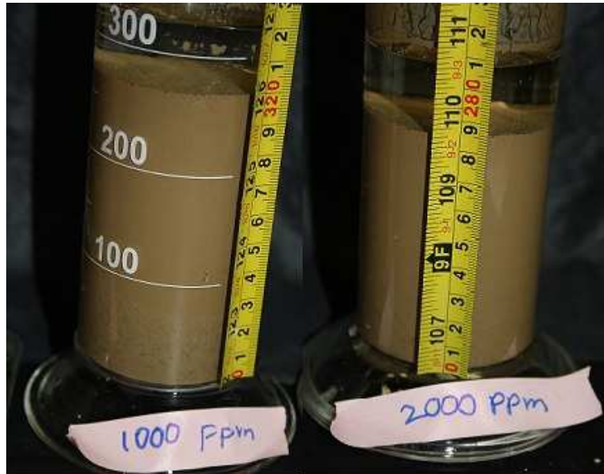
Figure 4.14: Settling columns (1000 ppm and 2000 ppm NaHCO_3 ) after 10 days
