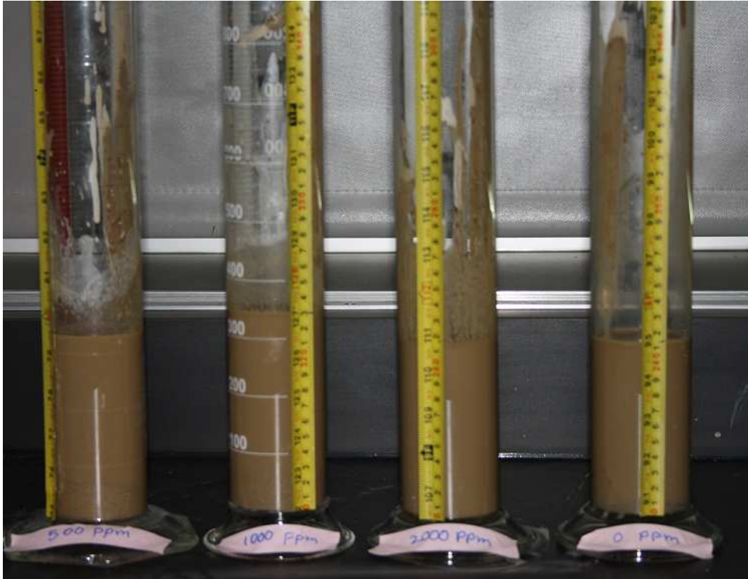
Figure 4.10: Settling columns with different sodium bicarbonate concentration (initial condition)
