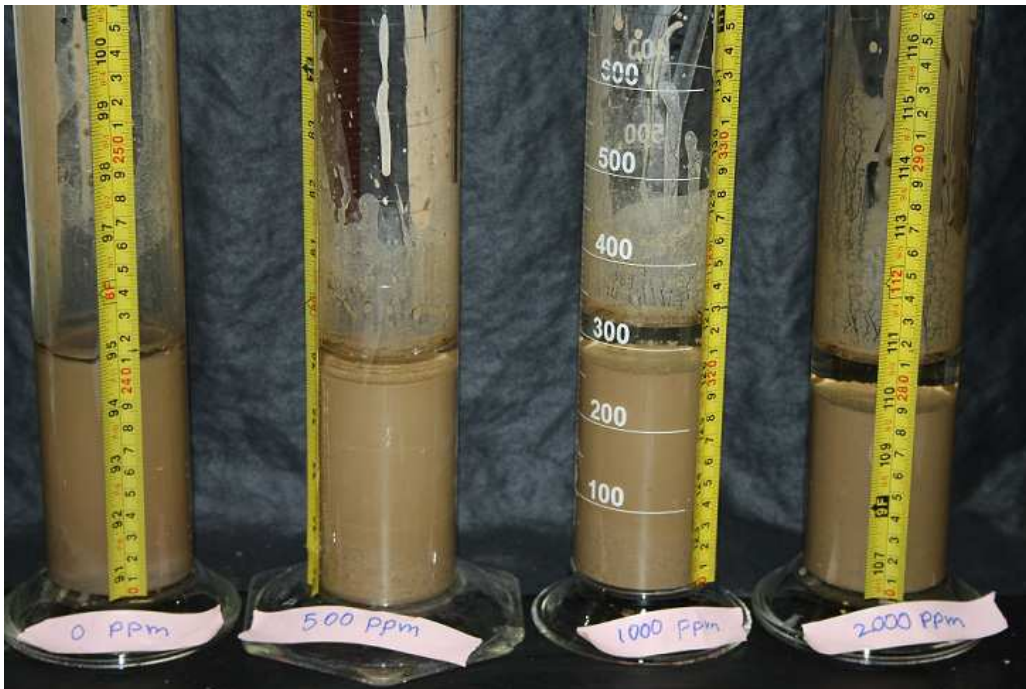
Figure 4.12: Settling columns with different sodium bicarbonate concentration (after 10 days)
