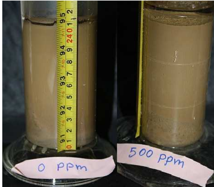
Figure 4.13: Settling columns (without and with 500 ppm NaHCO_3 ) after 10 days
