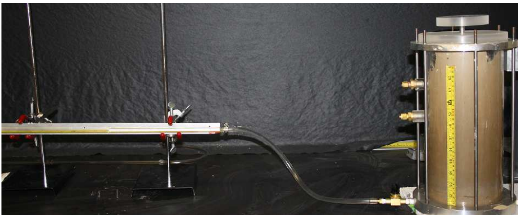
Figure 4.9: Consolidometer and hydraulic conductivity measurement setup
