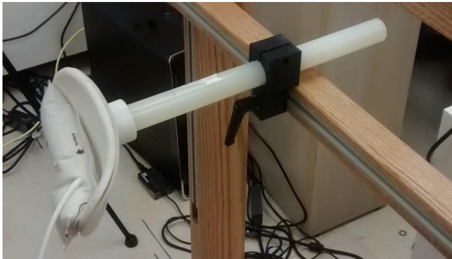
Figure 5-11. PCA mounted on crossbar
