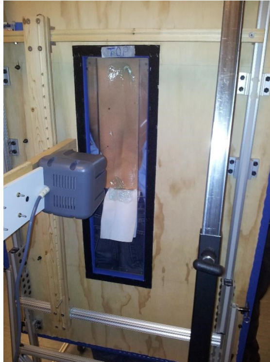
Figure 5-5. Back of old frame, demonstrating ultrasound access slot
