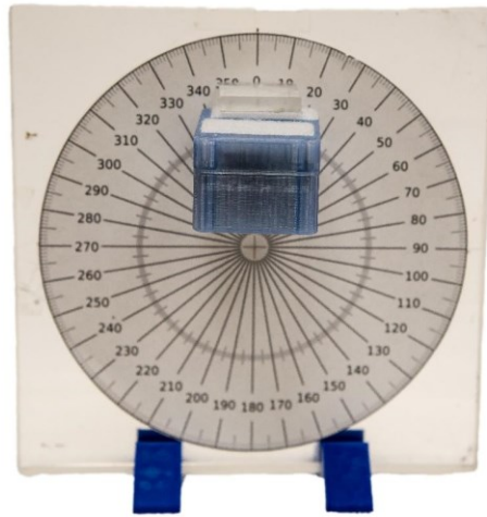
Figure 5-22. Rotating protractor with angle sensor attached
