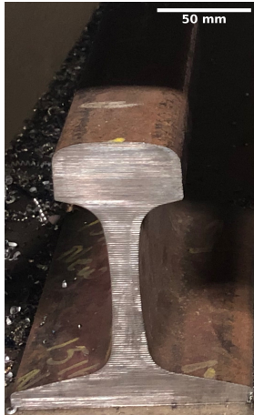
(a) As-received profile of the a commonly used 115 lb/yd Canadian rail steel (b) As-received profile of the a commonly used 136 lb/yd Canadian rail steel
