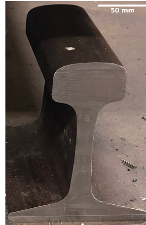
(a) As-received profile of the a commonly used 115 lb/yd Canadian rail steel (b) As-received profile of the a commonly used 136 lb/yd Canadian rail steel
