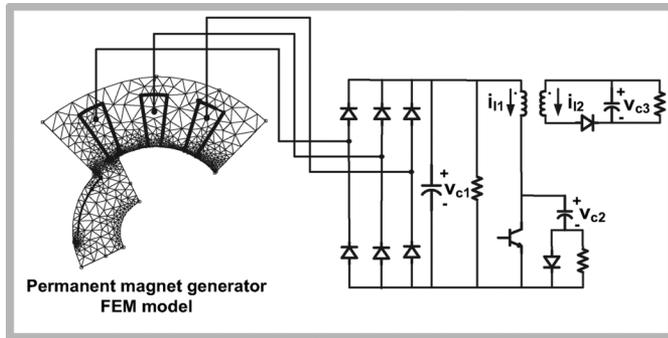
Fig. 5. PM generator feeding a flyback converter analyzed in [56], based on the SS approach for coupling.
