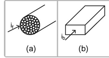
Fig. 1. (a) Stranded conductor. (b) Solid conductor.
