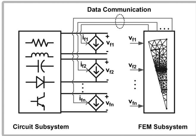
Fig. 6. Schematic of an indirectly coupled field-circuit system based on the current output approach.
