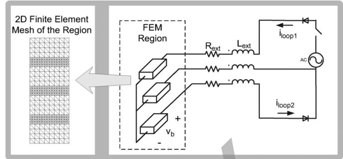
Fig. 2. System of three busbars in a rectangular domain studied in [20] and [21] based on the loop current method for coupling.
