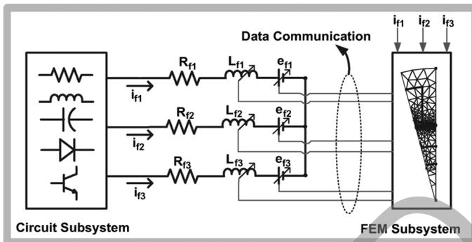
Fig. 7. Schematic of an indirectly coupled field circuit system based on the circuit parameter approach.
