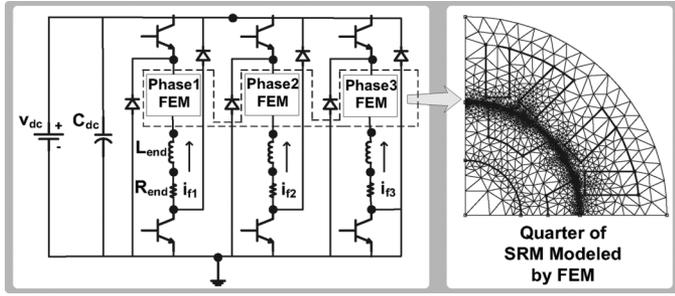
Fig. 4. Electric circuit and finite-element mesh of a switched reluctance motor analyzed in [39], based on the nodal approach for coupling.
