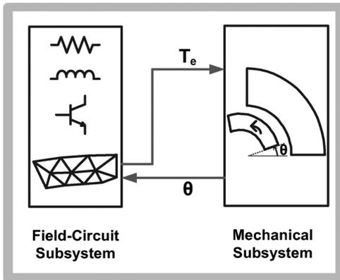
Fig. 8. Schematic of the iterative procedure between the field-circuit and mechanical subsystems.
