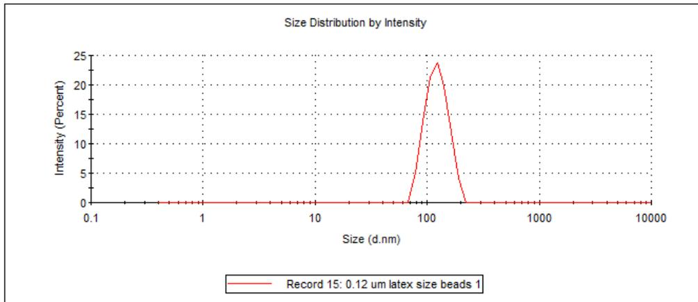
**Figure 4.2 Sizing result for 120 nm standard latex beads**
