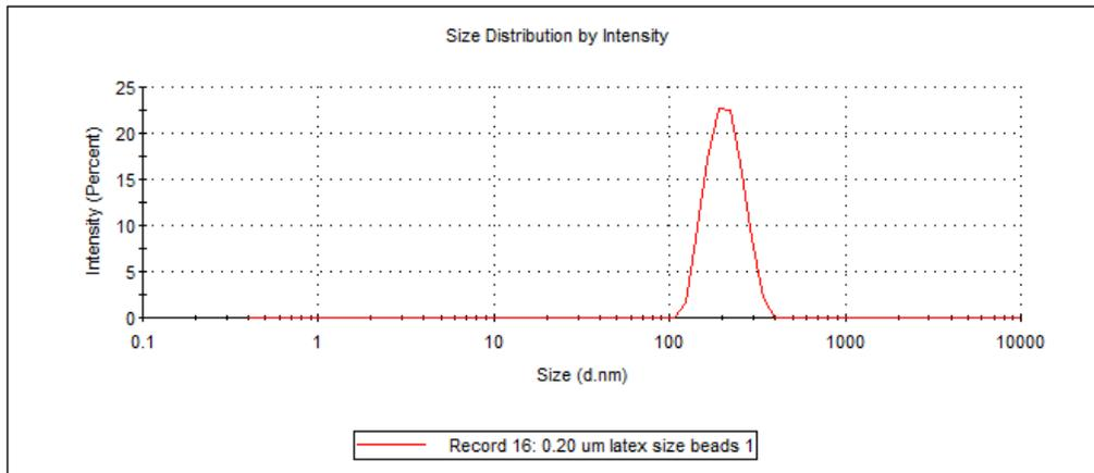
**Figure 4.3 Sizing result for 200 nm standard latex beads**
