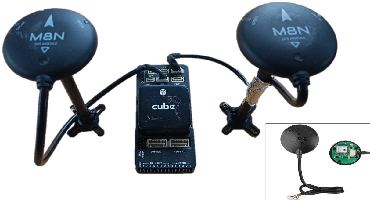
Figure 11. Interfaced module of two M8N receivers with Pixhawk Cube. Inset: GPS signal receiver M8N with a built-in BDS compass module and antenna.
