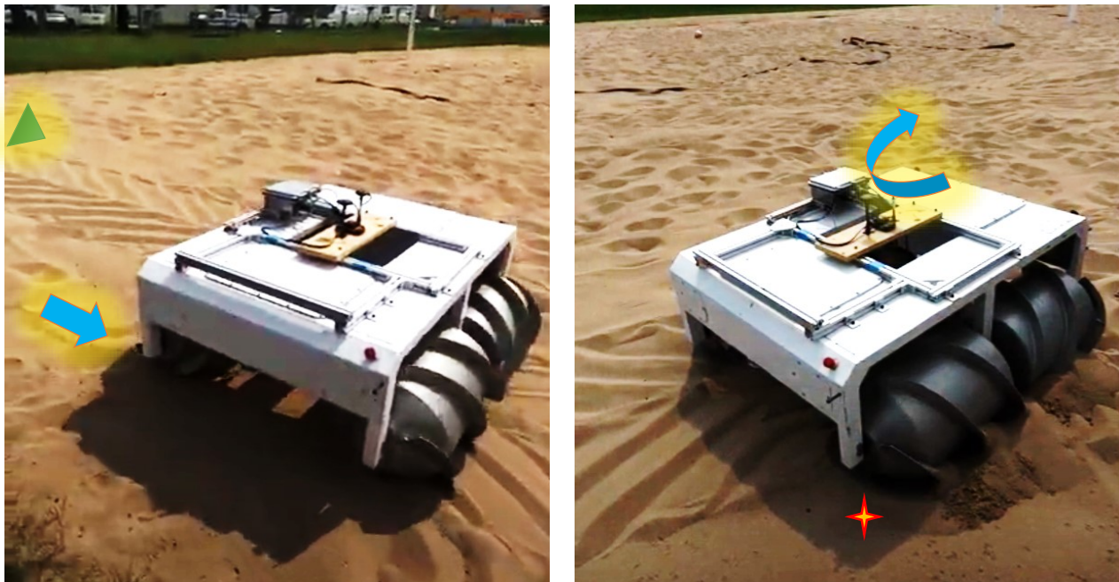
Figure 32. The results of scroll movement implementation in sand medium for a square trajectory: (a) Left image shows the start point and the direction of motion of rover along one edge of the square trajectory, (b) Right image shows the first waypoint out of the four waypoints at which the rover is expected to make a 90 degree turn on-spot to traverse along the adjacent edge of the trajectory.
