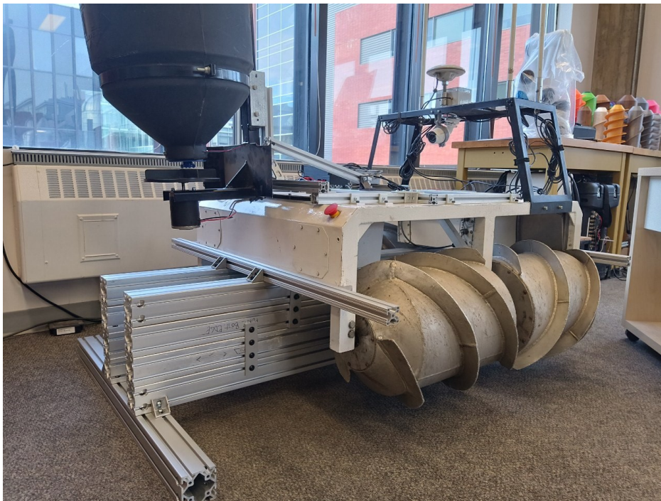
Figure 20. Fully Assembled Helix Rover on Block: The Helix rover, equipped with a comprehensive array of electronic components and hardware interfaces, stands ready for testing and experimentation in the controlled laboratory environment.
