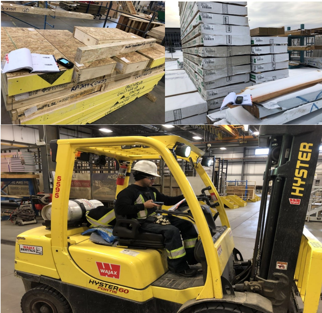
Figure 5-11. Implementation of Real-time Technology at ACQBUILT Plant Figure 5-11 shows a photograph of the operator transferring material from stock in the yard to the fabrication shop with the scanner in hand.
