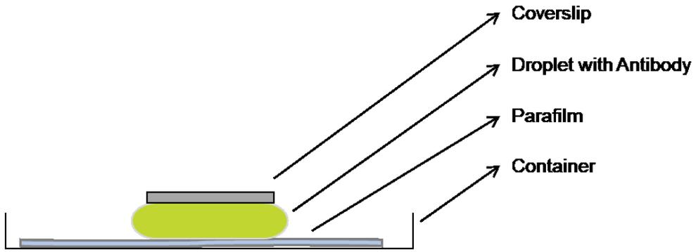
**Figure 4. Inverted Coverslip on Droplet Microscopy Method.**
