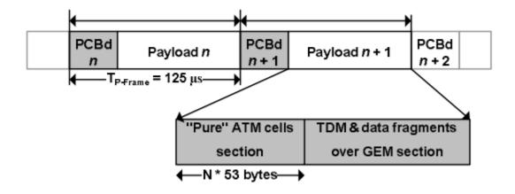
The frame is 125 µm for both downstream data rates. The PCBd length range is the same for both speeds and depends on the number of allocation structures per frame. If there is no data for sending, downstream frame is still transmitted and used for time synchronization.
