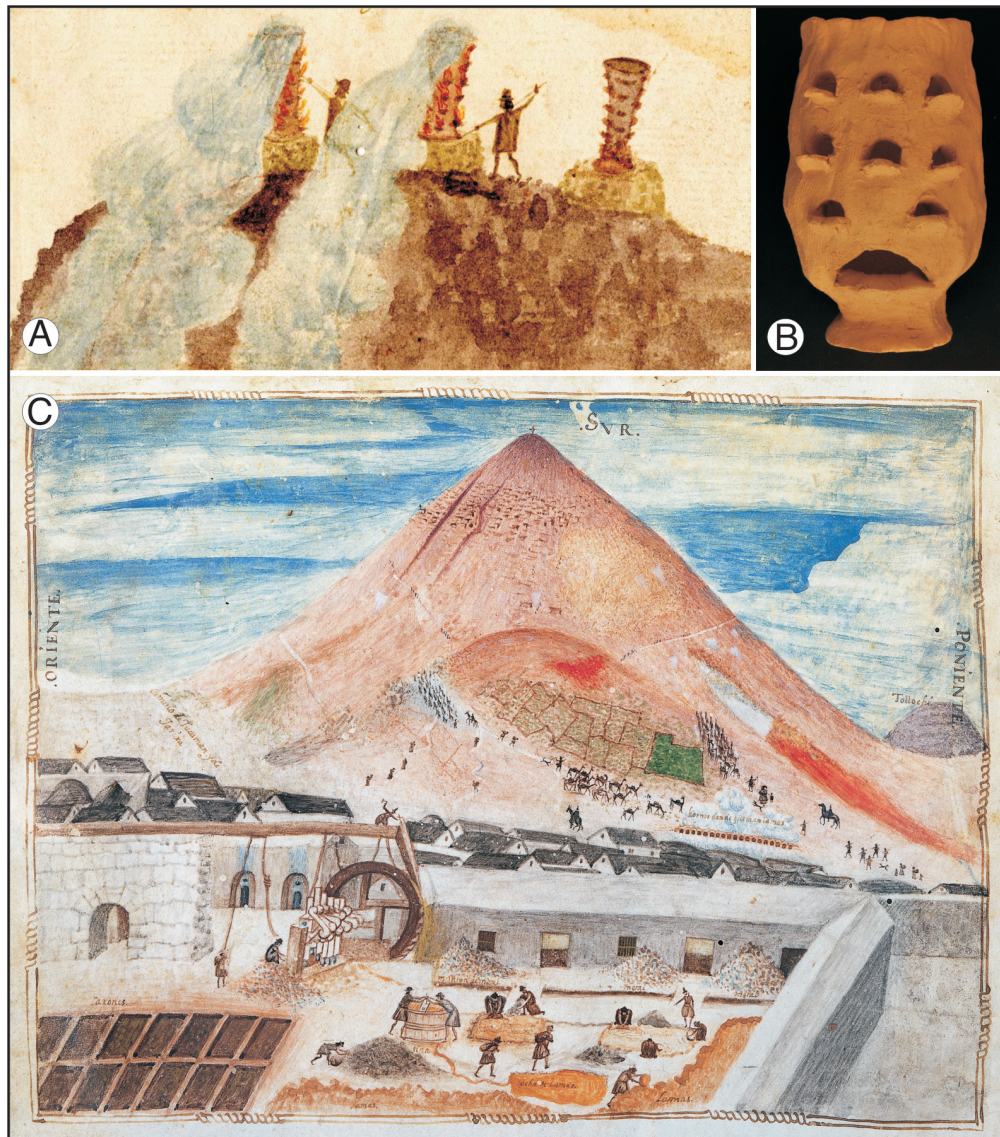
Fig. 4.2. (A) Painting from the Colonial era of smelting operations at Cerro Rico de Potosí using Incan huyaras (artist unknown). (B) Model of a clay huyara used to smelt argentiferous ores at the time of Colonial contact. The small slots vented the kiln, whereas the molten metal was retrieved from the large basal opening. Ore was introduced from above, onto the fuel. The model was created by the late Jeanne M. Wolfe (McGill University). (C) A 1584 painting by an unknown artist of Cerro Rico de Potosí, with trains of llamas transporting ore from the mountain to one of the amalgamation facilities built to process the ore. The paintings are courtesy of The Hispanic Society of America .
