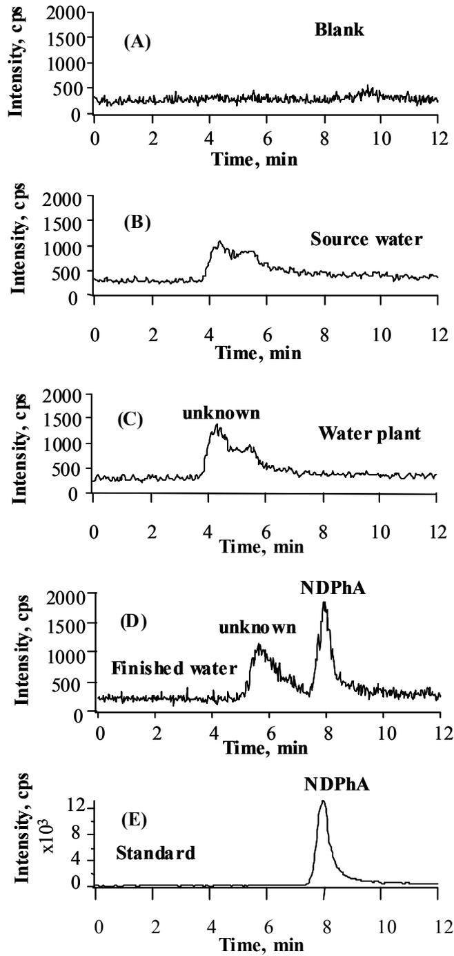
**Figure 2.5: Determination of NDPhA in (A) blank, (B) source water, (C) treated water sample collected from the water treatment plant, (D) treated water sample collected from a location in the distribution system, and (E) NDPhA standard.**
