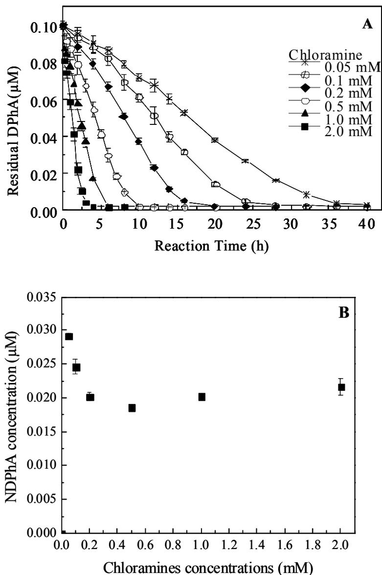
**Figure 5.8: Effect of initial chloramine concentration on NDPPhA formation from DPhA. (A) Residual DPhA concentration after reacting with different chloramine concentrations over time; (B) NDPPhA concentrations produced at equilibrium from different initial chloramine concentrations.**
