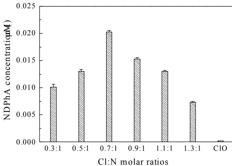
**Figure 5.9: Effect of Cl:N ratio on NDPhA formation from DPhA (0.1 $\mu$ M) after 12 h.**
