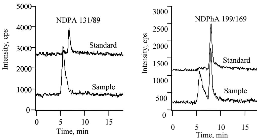
**Figure 2.2: MRM chromatograms of a standard spiked Optima water extract and a drinking water sample showing the separation of NDPA and NDPhA from background interference. The standard concentration in the spiked Optima water sample was 5 ng/L of each nitrosamine.**
