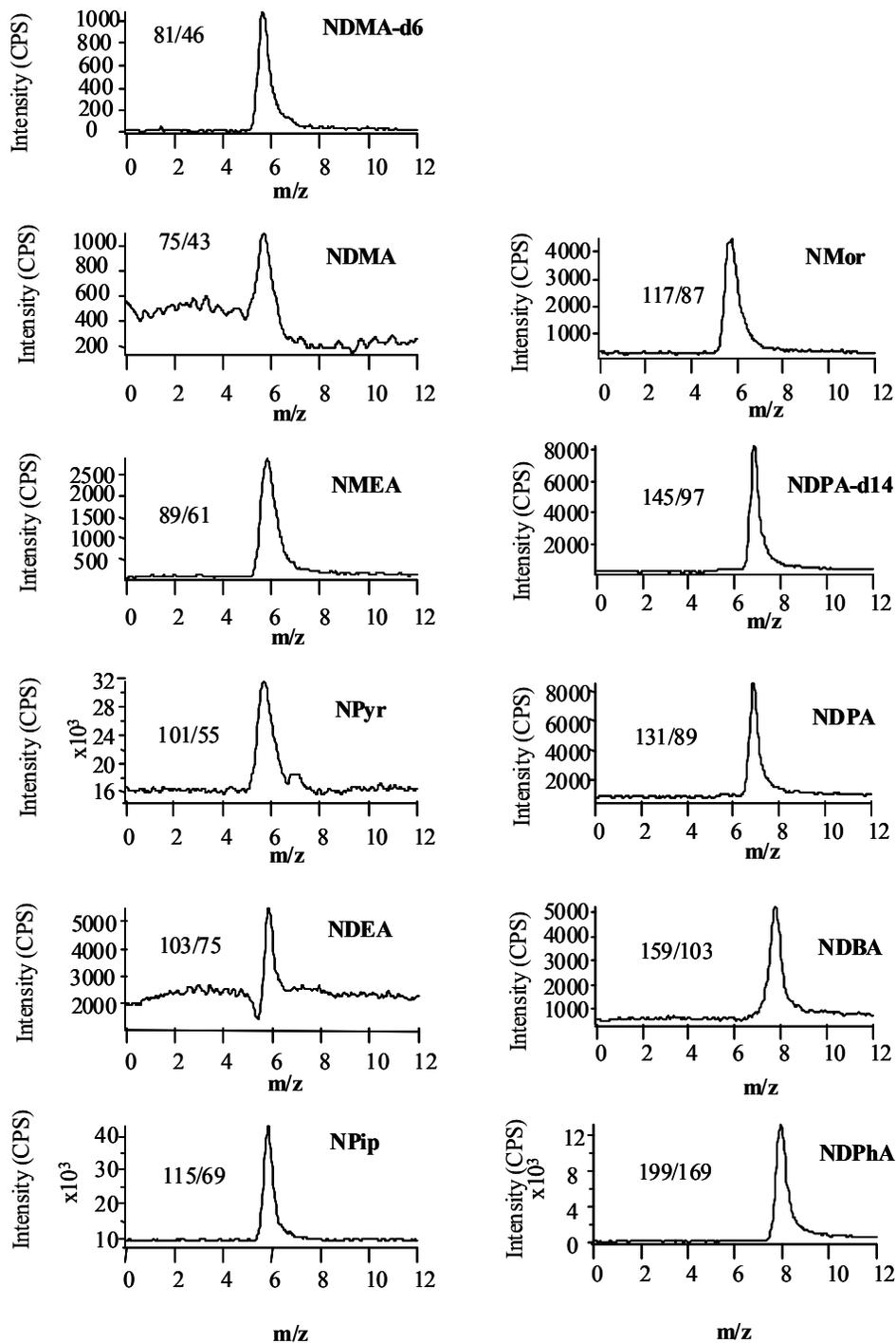
**Figure 2.3: Chromatograms of the nine nitrosamines obtained from an Optima water sample spiked with the nine standards and two internal standards under the optimized conditions.**
