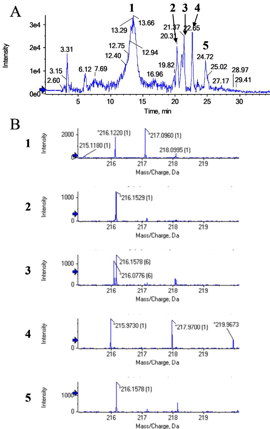
**Figure 6.6: TripleTOF analysis of chlorinated *P. fluorescens* extracts. (A) XIC of 217.0 +/- 1.0 Da (B) MS spectra of peaks 1–5 focused on m/z 214.0–220.0.**
