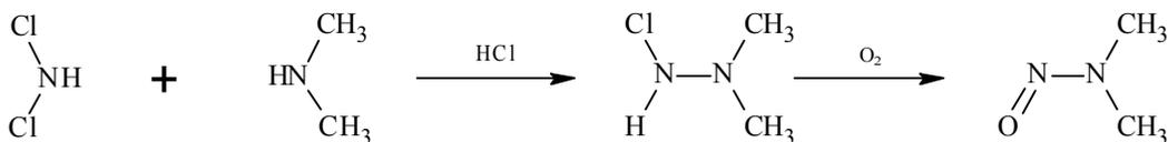
**Figure 5.1: Proposed mechanism for the formation of NDMA from DMA and dichloramine. From [5, 6].**
