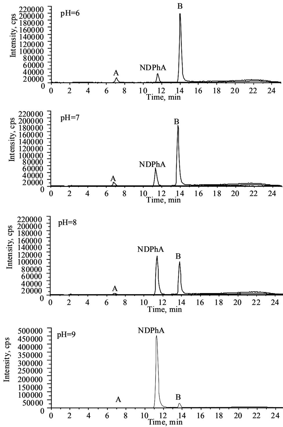
**Figure 5.12: MRM chromatograms of Peaks A and B and NDPhA produced at pH 6–9. Sample prepared by reacting 0.1  $\mu$ M DPhA with 1.0 mM chloramines at pH 6–9.**
