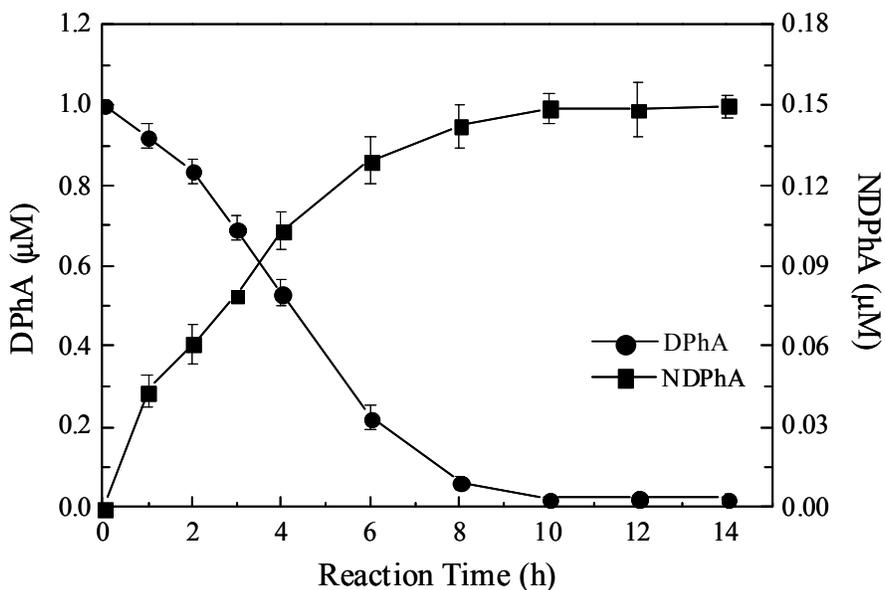
**Figure 5.6: Time course of NDPhA formation from the reaction of 1.0  $\mu\text{M}$  DPhA with 1.0 mM chloramines.**
