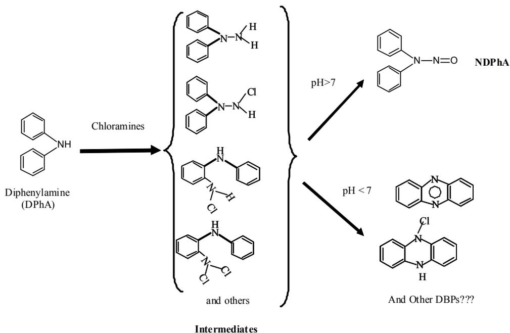
**Figure 5.14: Putative pathways for the formation of NDPhA and other N-DBPs from chloramination of water containing DPhA**
