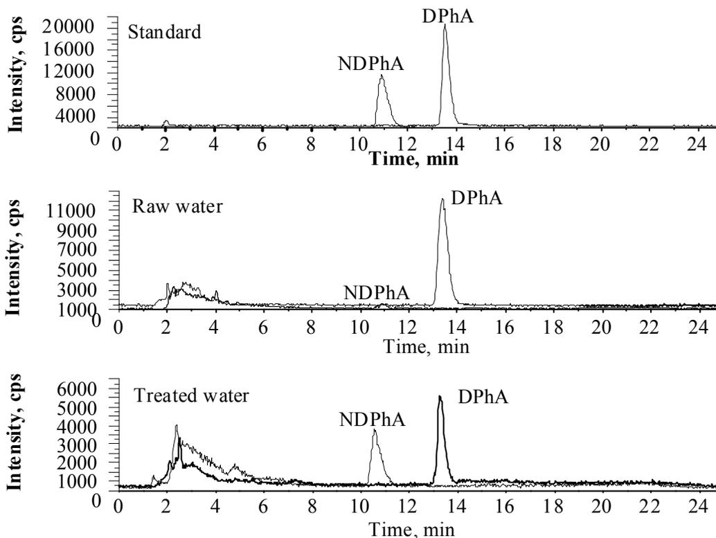
**Figure 5.5: LC-MS/MS analysis of DPhA and NDPhA in standards, raw water, and chloraminated water.**
