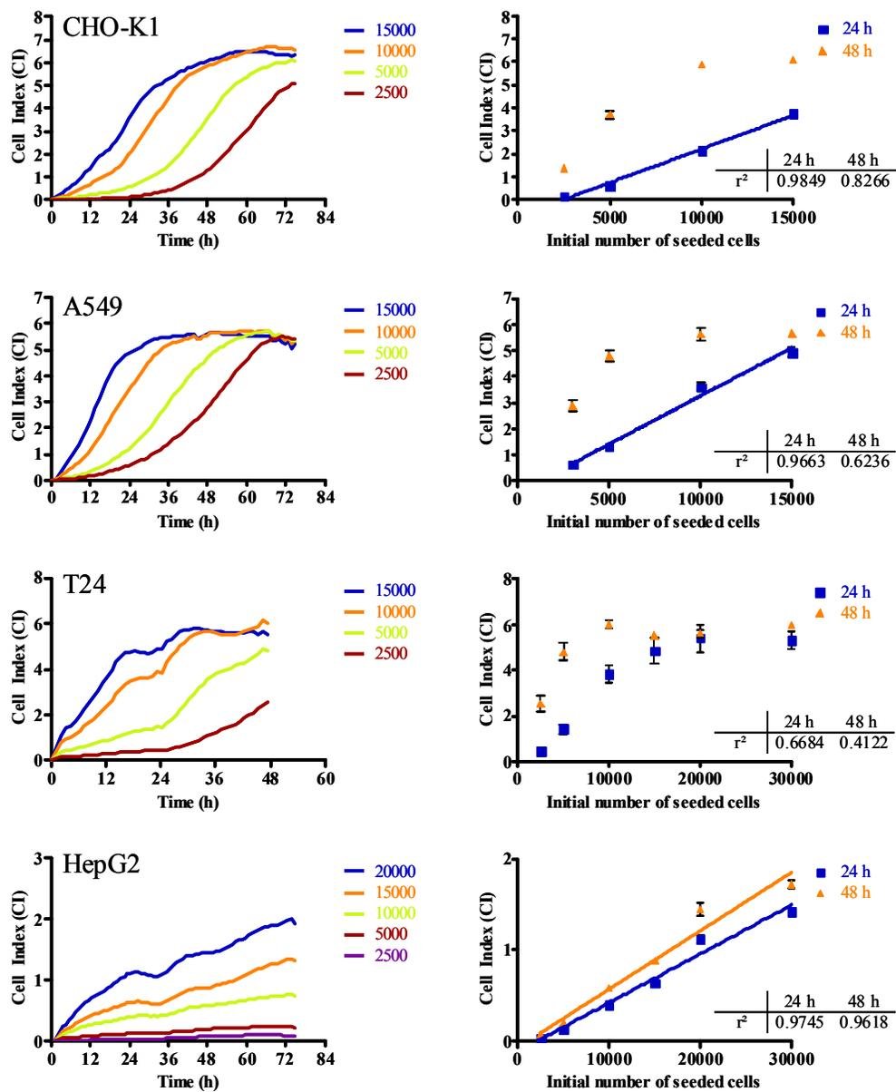
**Figure 4.1: RT-CES curves and linear relationship between cell index (CI) and initial number of seeded cells. The linear relationships between RT-CES CI and the number of seeding cells are found during the log phase.**
