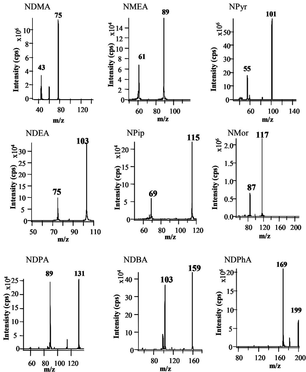
**Figure 2.1: MS/MS spectra of the nine nitrosamines showing their parent ion and characteristic product ion.**
