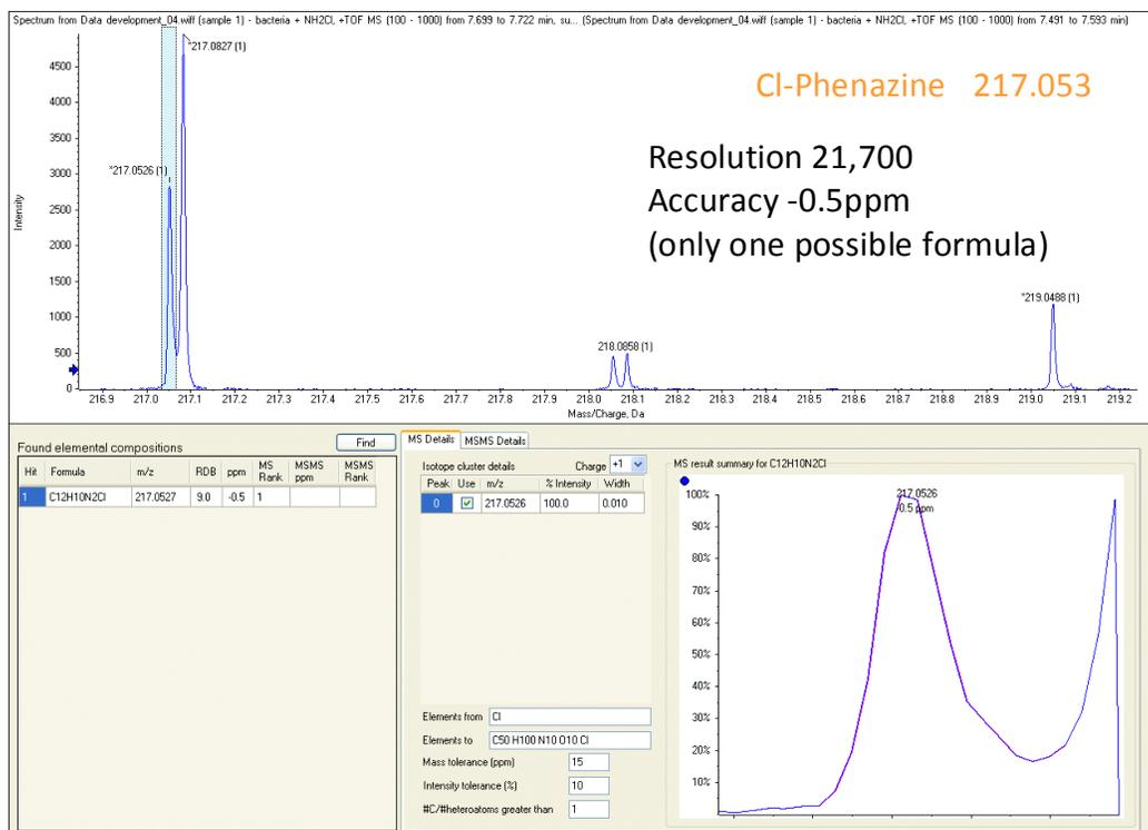
**Figure 6.2: Accurate mass analysis of suspected N-chlorophenazine peak in a chloraminated *Pseudomonas fluorescens* sample.**
