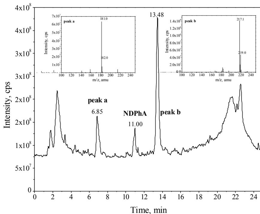
**Figure 5.11: LC-MS total ion chromatogram of a chloraminated DPhA extract (pH 7). Inset A: EMS spectra of peak A. Inset B: EMS spectra of peak B. Sample prepared by reacting 0.1  $\mu\text{M}$  DPhA with 1.0 mM chloramines at pH 7. After reaching equilibrium the reaction mixture was extracted and analyzed using LC-MS with enhanced scan mode.**
