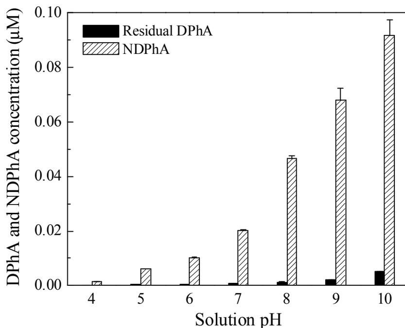
**Figure 5.10: Effect of pH on NDPPhA formation and residual DPhA concentration. DPhA (0.1 µM) was reacted with 1.0 mM chloramines at pH 4, 5, 6, 7, 8, 9, and 10 for 6 h.**
