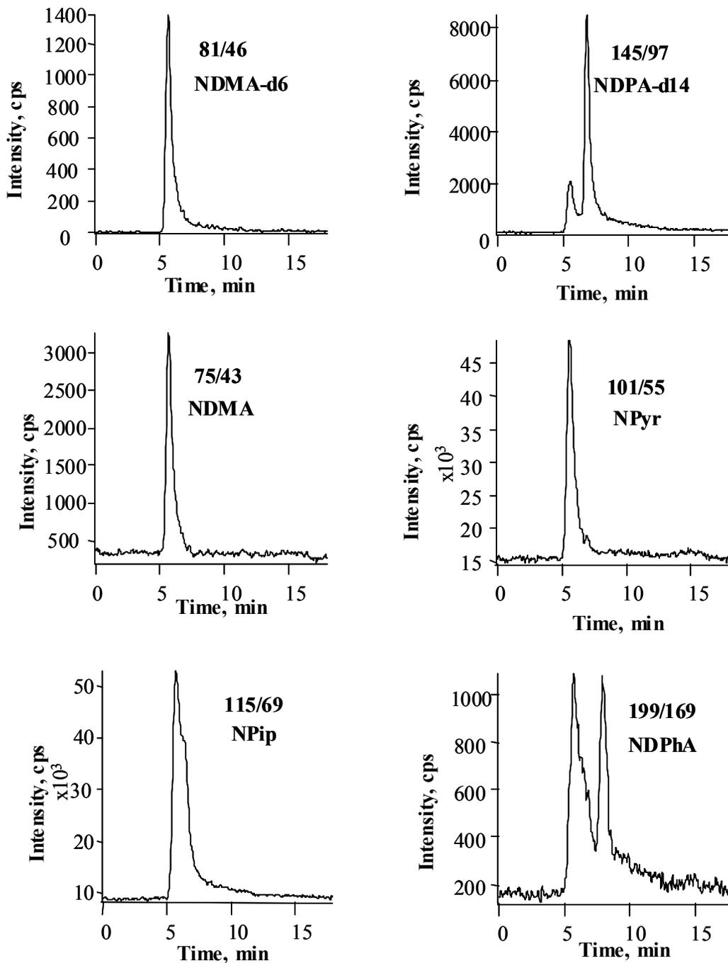
**Figure 2.4: Detection of NDMA, NPip, NPyr and NDPhA in a treated drinking water sample collected from a drinking water distribution system.**
