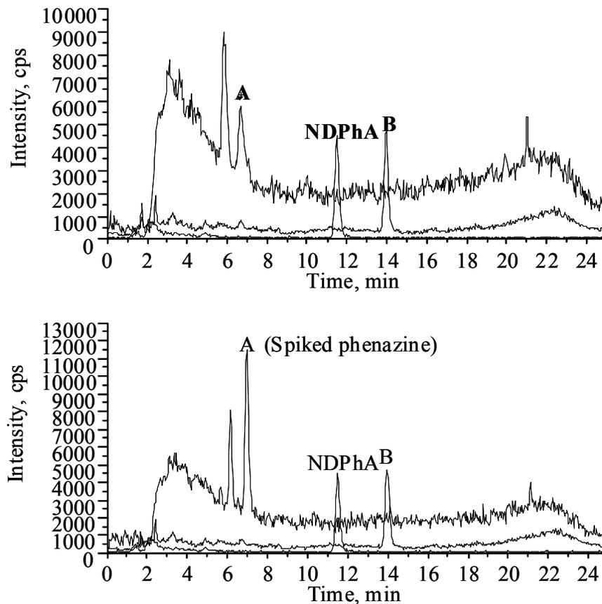
**Figure 5.13: MRM chromatograms of NDPhA, Peak A (phenazine), and Peak B (N-chlorophenazine) in chloraminated raw water.**
