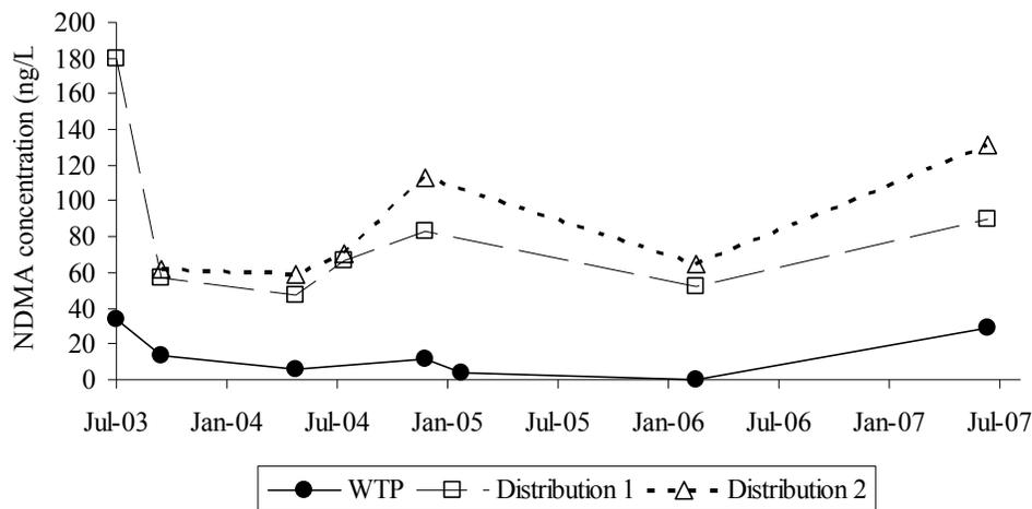
**Figure 3.1: NDMA concentrations detected in water samples collected from System 1 between 2003 and 2007. Distribution 2 is farther away than Distribution 1 from the water treatment plant.**
