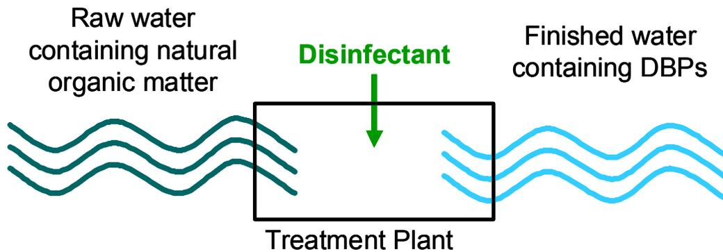
**Figure 1.1: Schematic of disinfection byproduct formation during water treatment.**
