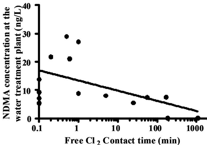
**Figure 3.2: Effect of free chlorine contact time on NDMA concentrations produced by chloramine disinfection. NDMA concentrations are from treated water samples collected at the water treatment plant. The line indicates a trend.**
