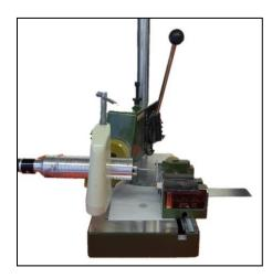
**Figure 6.39** Custom microsampling system created for this study. A Proxxon Micromet drill stand is equipped with a Proxxon Machine (micro) vise with self-stick non-slip surface grip pads. A Dremel precision rotary tool equipped with a diamond cut wheel (0.15 mm thickness) is clamped onto the drill stand. System serves as a Dremel-equipped miter saw (Bishop *et al.*, 2020).
