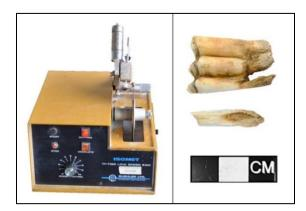
Figure 6.38Anterior lobe separation for sample SG03.Left: Isomet 1-1180 low speed precision cutter with LM3 clamped for processing.Right: LM3 post-cutting, showing the anterior lobe removed from the main tooth.
