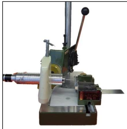
**Figure 6.39** Custom microsampling system created for this study.
