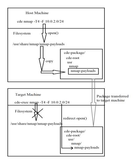
Since only the files that were accessed during the execution of the program are captured, it can only provide the functions on the executed program path. CDE memory also creates paths to file system which has no files since some programs check for such paths/libraries while they are being launched to do initial check. This way the virtualized package does not go into run-time errors.
