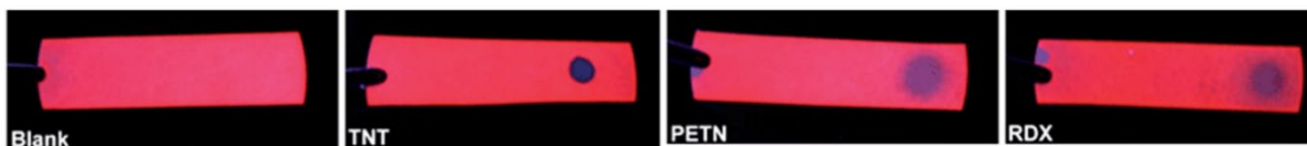
Figure 1-18. Detection of the high-energy compounds TNT, PETN, and RDX using red-photoluminescent SiQDs immobilized on filter paper. The images were taken while the paper sensors were exposed to a handheld UV lamp. Adapted with permission from M. Gonzalez, C.; Iqbal, M.; Dasog, M.; G. Piercey, D.; Lockwood, R.; M. Klapötke, T.; C. Veinot, J. G. C. Nanoscale 2014 , 6 (5), 2608–2612. Copyright © 2014 Royal Society of Chemistry.
