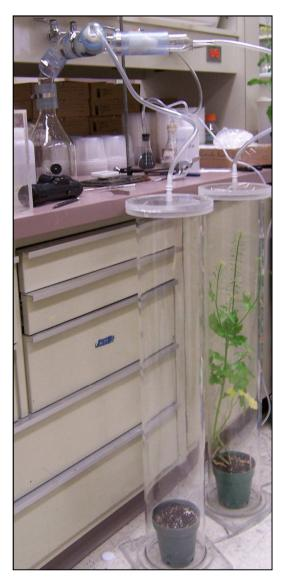
Figure 4.1. Y-tube olfactometer.
