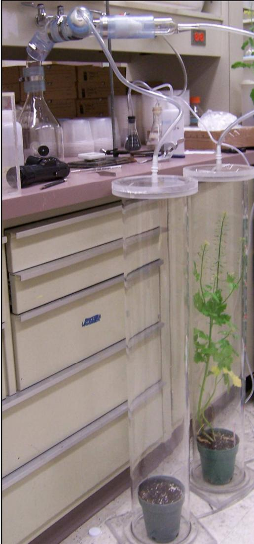
Figure 4.1. Y-tube olfactometer.
