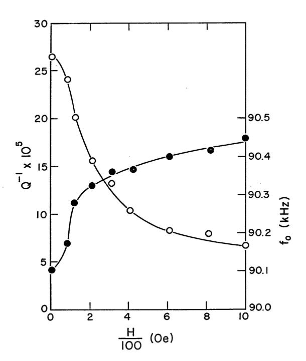
The low temperature magnetic damping observed here closely resembles the so called "plateau region" in the temperature dependence of Q<sup>-1</sup> in iron, which was first observed by Bruner (1959) and Heller (1961). Investigations of this plateau have been reported by Vienneau (1968) and by Verdini and Vienneau (1968 a). (See Section D of this Chapter, dealing with magnetic damping in iron.)
