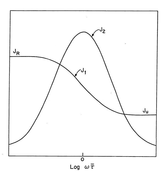
The internal friction, tan  $\phi$ , given by equation (2.9) has a maximum at  $\omega\tau$  = 1, given by:
