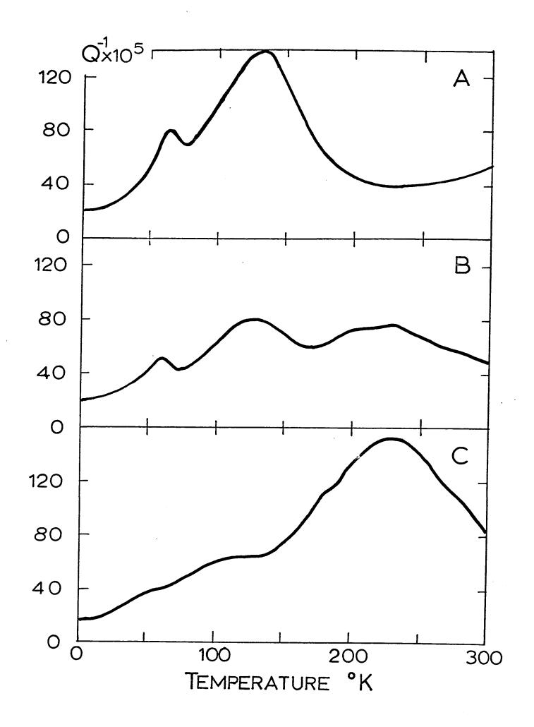
THE EFFECT OF INCREASING COLD WORK ON THE  ${\rm P_3~PEAK~IN~NICKEL~(f~\approx~20~kH_{_{\bf Z}})}$
