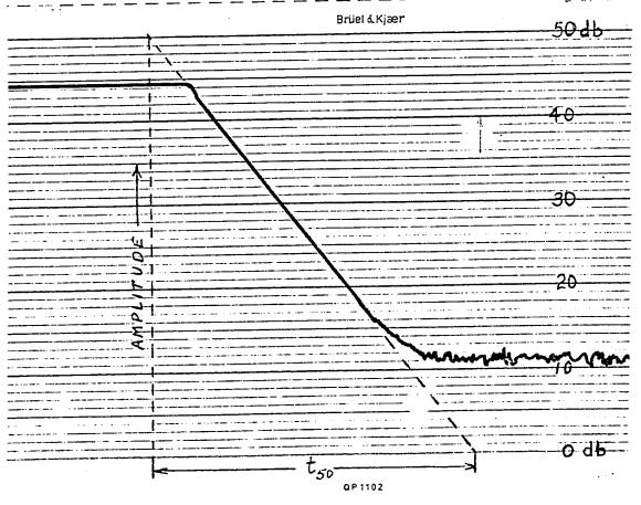
of time on the logarithmic level recorder following cut-off of the driving voltage. The trace of a typical decay is shown in figure 3.4(b). The exponential decay produced a straight line which could be extrapolated to 50 db to arrive at the time  $t_{50}$ . After measurement of the resonant frequency, the internal friction was evaluated from:
