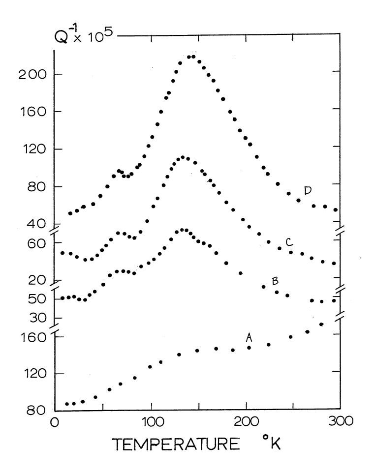
the  $Q^{-1}$  curve at about  $140^{\circ}K$ . This is accompanied by a smaller peak (to be called  $P_2$ ) in the vicinity of  $65^{\circ}K$ . A fourth very interesting effect of cold working is the clearly visible increase in  $Q^{-1}$  as the temperature is lowered below  $50^{\circ}K$  for 3% and 5% deformations. This is in contrast to the well-annealed and the slightly cold worked cases where  $Q^{-1}$  continuously decreases as the temperature is lowered.
