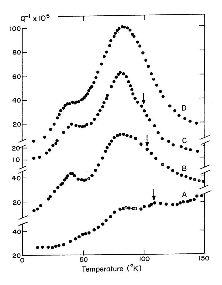
relaxation peak characterized by a single limiting relaxation time and a spectrum of activation energies whose width is given by equation (4.3). It has also been observed that at least three peaks remain distinct from the main peak for deformations as large as 25%, and exhibit themselves as the so called Niblett-Wilks peak.
