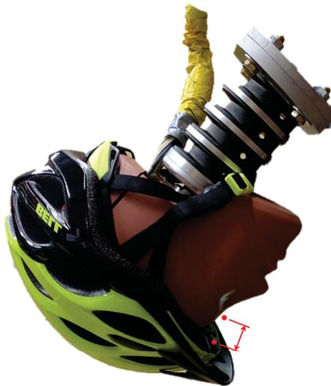
Figure 4.1: Head Helmet Displacement Vector
