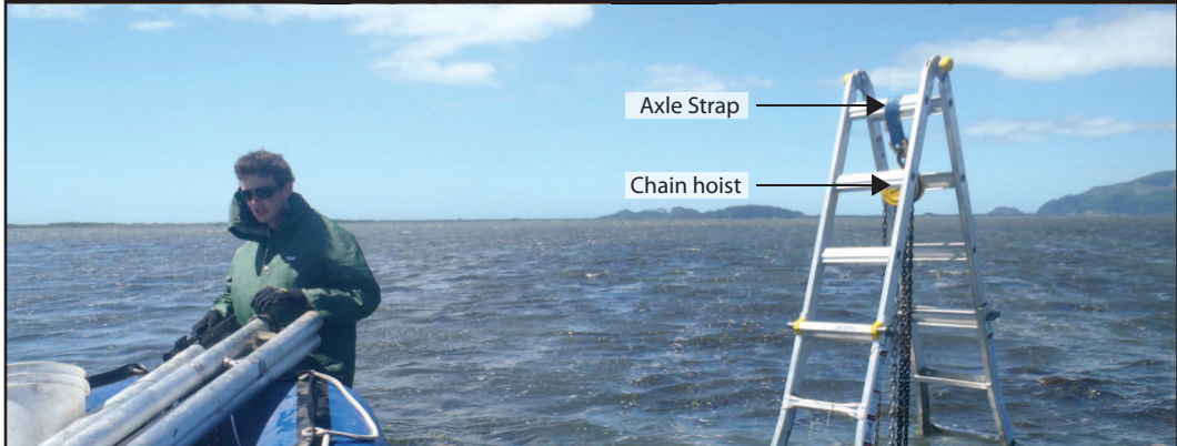
Figure 1-8. Vibracoring method and equipment. Top and center photos: Dave attaching an aluminum pipe to the pipe clamp. Once that step is complete, the pipe is raised into place over the sediment. The motor of the wheelbarrow-mounted cement shaker, once started, transmits high-frequency vibrations through the flexible hose, through the pipe clamp, and to the pipe itself. This process advances the pipe into the sediment. To retrieve the pipe, the ladder is placed over it; a chain is then wrapped around the exposed top of the pipe, and its ends are attached to the hook on the chain hoist, used to pull the pipe out of the sediment. Bottom photo: vibracoring in shallow water.
