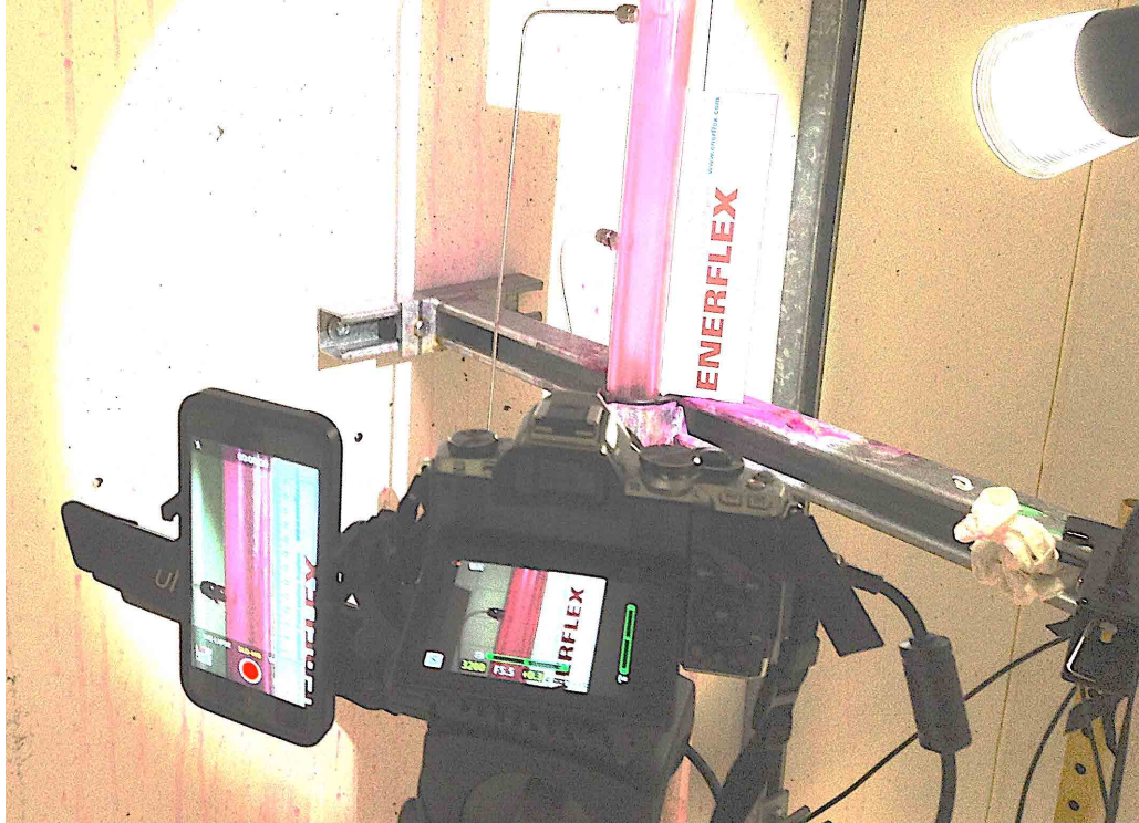
Figure 3.14 iPhone 6s (L) and Olympus DSLR (R) Mounted for Imaging.
