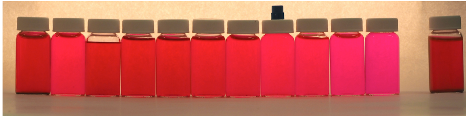
Figure 3.19 Comparison of Flow Loop Rhodamine Sample vs. Prepared Concentrations. (Flow loop sample is marked with black plastic on top.)
