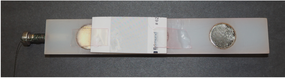
Figure 3.17 Calibration Target Mounted to Target Holder.
