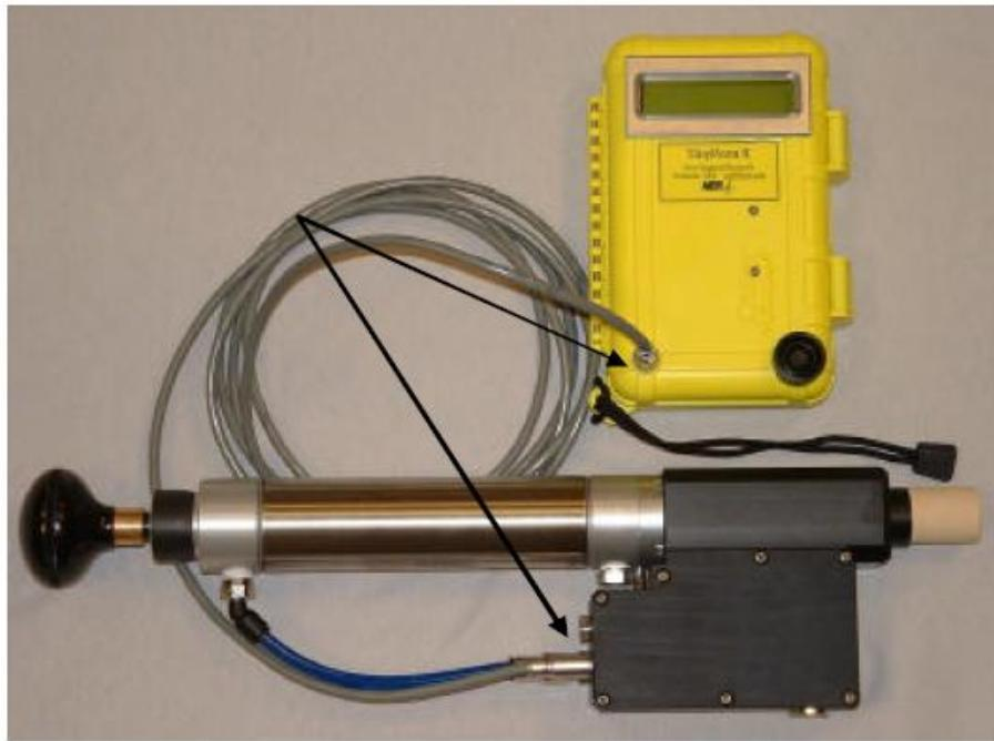
**Figure 5.4: Tiny Perm II, the portable air permeameter system used in measuring the air permeability of our samples. The two arrows are pointing out the connection between the pressure transducer in the black box to the yellow microprocessor and control unit.**
