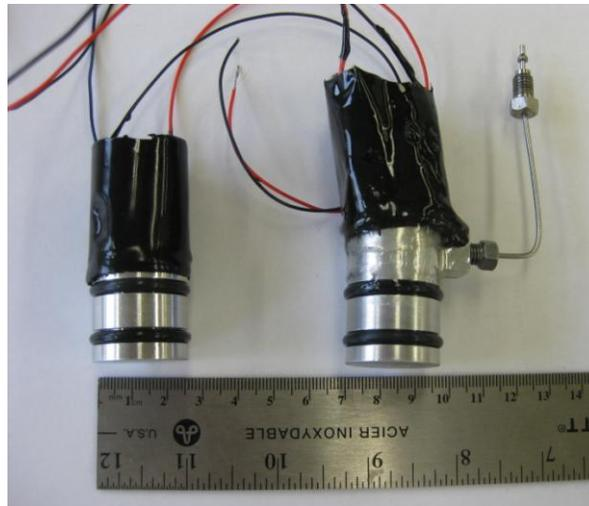
**Figure 4.2: (top) Cartoon depiction of the various components in a transducer. (bottom) A photography of a completed pair of transducers (pulser and receiver). The transducer on the right has the pore pressure inlet.**
