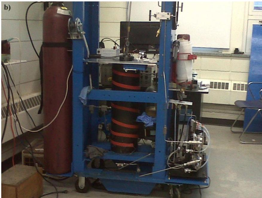
**Figure 4.4: a) A simplified schematic of the experimental set up. b) Photograph of the laboratory equipment used. The acquisition system behind the pressure vessel and is not captured in the photograph.**
