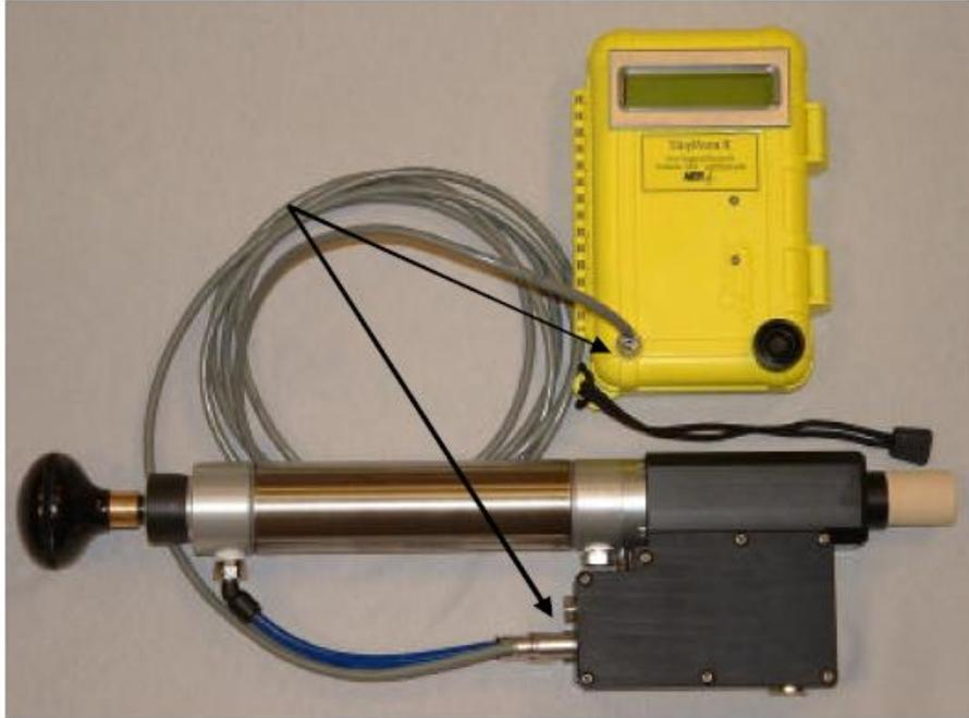
**Figure 5.4: Tiny Perm II, the portable air permeameter system used in measuring the air permeability of our samples. The two arrows are pointing out the connection between the pressure transducer in the black box to the yellow microprocessor and control unit. Photograph from NER Tiny Perm II user's manual.**
