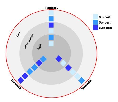
Figure 2 - 2. Schematic diagram (not to scale) of  $1 \times 1$  m peat plots at three positions relative to the water table present on each of four clay islands. Peat placed in "low" plots were submerged at the start of the study. Plots located in the "intermediate" position were located very near to or just above the water table, and plots in the "high" position were entirely above the water table.
