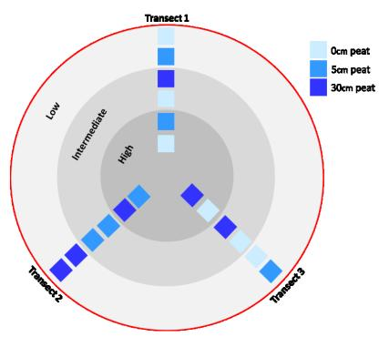
Figure 3 - 2. Schematic diagram of 1 x 1 m plots at three positions relative to the water table present on each of four clay islands. Plots in the "low" position were submerged at the start of the study. Plots located in the "intermediate" position were located very near to, or just above the water table, and plots in the "high" position were entirely above the water table.
