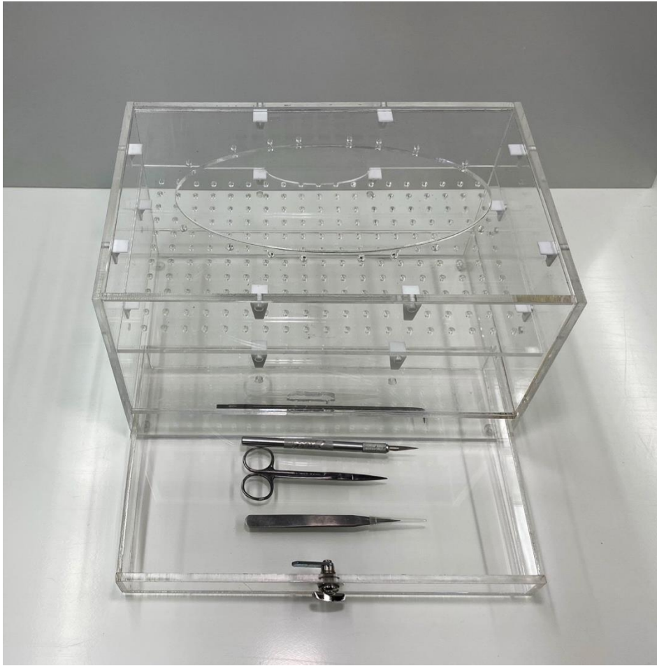
Figure 7. 2: Final plexiglass model. Board is positioned at the second level of depth and the largest lid size is shown.
