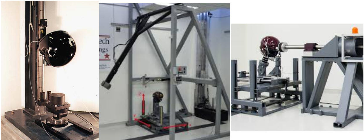
Figure 1.1: Linear drop test (left), pendulum impactor (center), and linear impactor (right) testing methods [10–12].
