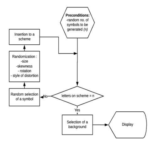
*Figure 5.* The scheme of the proposed CAPTCHA algorithm (Ogiela et al., 2018)
