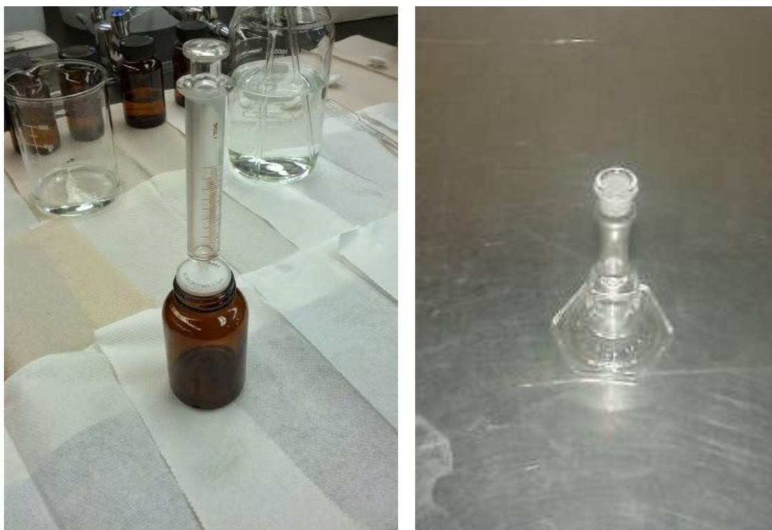
Figure A9. Glass syringe and 5 mL volumetric flask used in syringe adsorption test.
