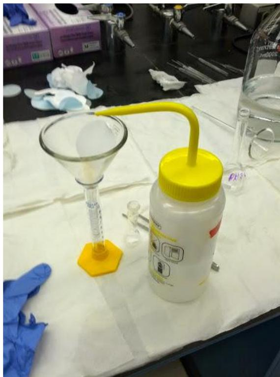
Figure A7. Filter membranes were rinsed by 50% phosphate-methanol solution (after NA adsorption) to the final volume of 5 mL. To do this, the filter membrane was transferred by forceps from glass bottles to glass funnel and rinsed. The solution was collected in 10 mL graduated cylinder and transferred quantitatively to 5 mL volumetric flask.
