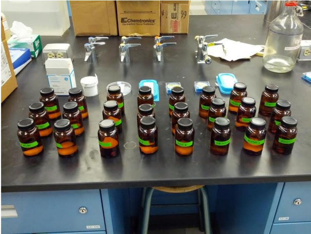
Figure A6. Filter membrane adsorption test (stationary phase experiment). Filter membranes were exposed to water sample in 125 mL glass (Type III soda-lime) bottles with black phenolic caps and PTFE/LDPE liner.
