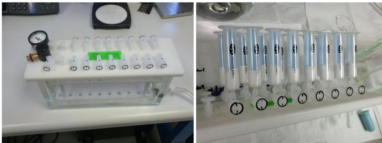
Figure A10. Extraction Manifold for solid phase extraction (SPE) and industrial resins experiments.
