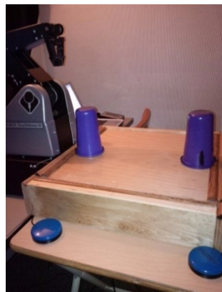
Figure 4-2 Platform and Robot set-up showing the two containers in position on the platform and the two participant switches used to control the robot arm.
