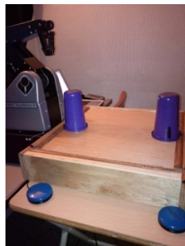
Figure 5-2 Platform and Robot set-up showing the two containers in position on the platform and the two participant switches used to control the robot arm.
