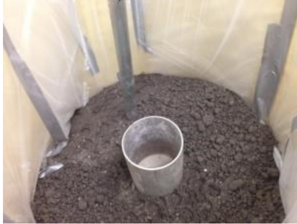
Figure 6-6 Compacting soil in different layers in jet grouting tank
