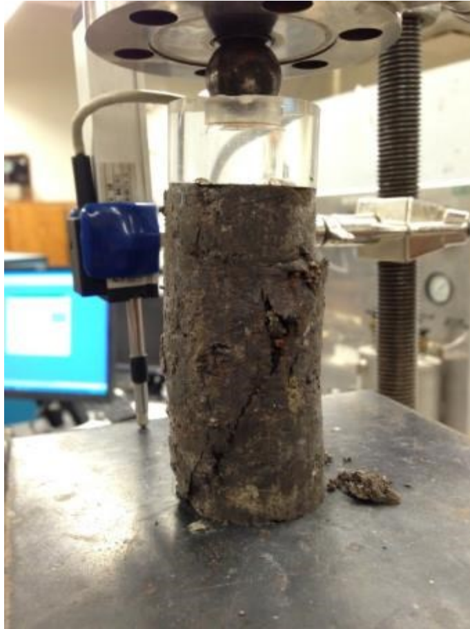
Figure 6-9 Uniaxial compression strength on reconstructed soil specimens
