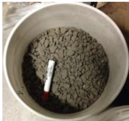
Figure 5-4 Maximum particle size of soil after crushing, 2cm
