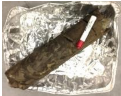
Figure 5-2 Extracted soil sample from core barrels
