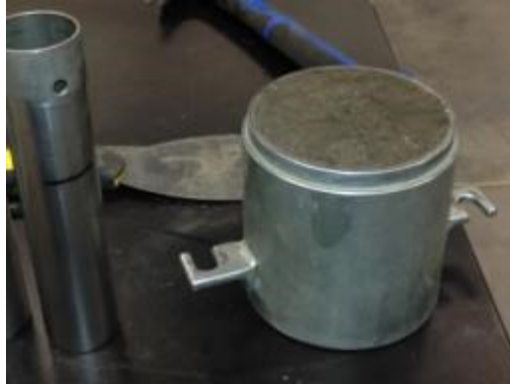
Figure 5-18 Compacted soil samples
