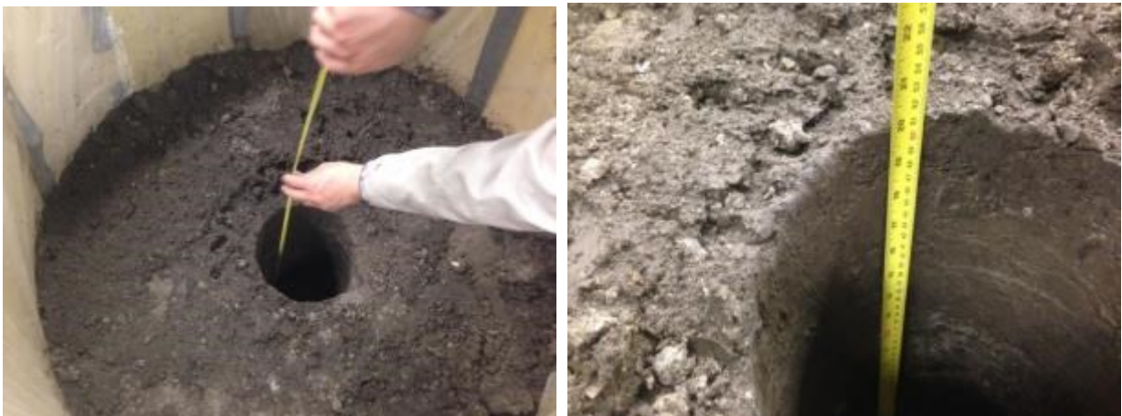
Figure 6-8 Reconstructed soil with a center jetting hole in jet grouting tank
