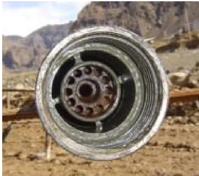
Figure 4-8 Triple-duck cross section of triple fluid jet grouting rod
