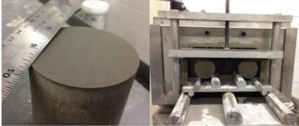
Figure 5-41 Grinding the top and bottom of the specimens
