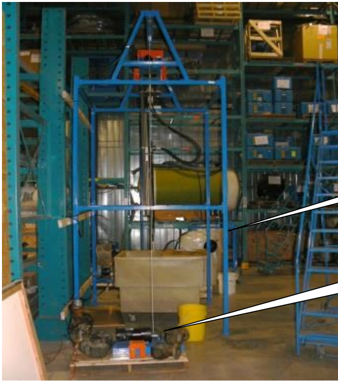
Figure 4-29 Vertical motion motor position and orientation
