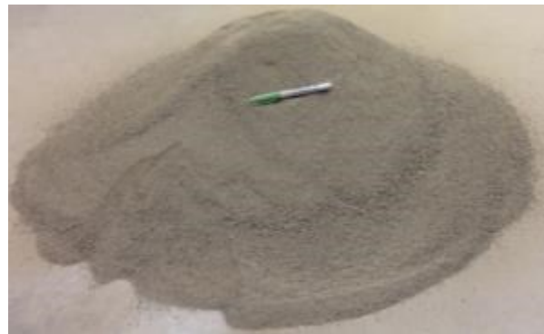
Figure 5-7 Mixing all grinded soil samples together
