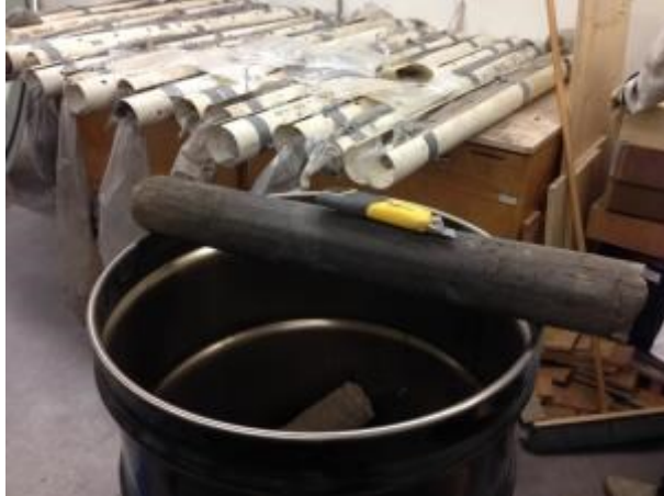
Figure 6-1 In-situ cores used to create reconstructed soil in laboratory
