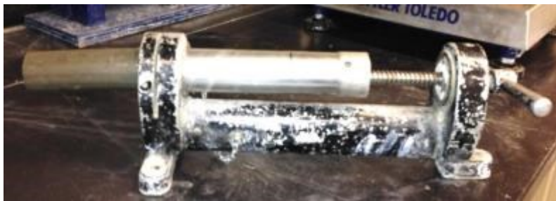
Figure 5-22 Extracting soil samples from Shelby tubes
