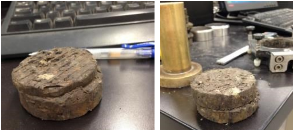
Figure 6-12 Direct shear test on reconstructed soil specimens
