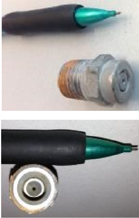
Figure 4-25 PW nozzles with smaller orifice sizes
