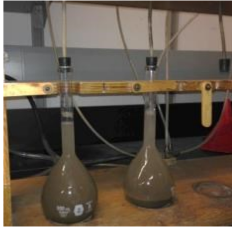
Figure 5-15 Specific gravity test
