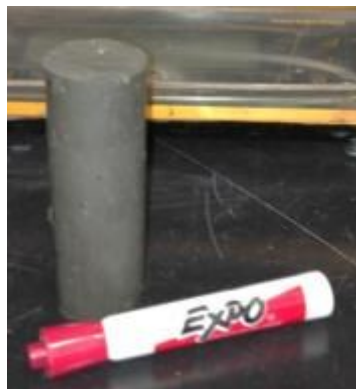
Figure 5-23 Soil sample for UCS test
