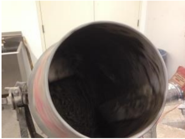
Figure 6-4 Conditioning oven dried and crushed soil with its in-situ moisture content
