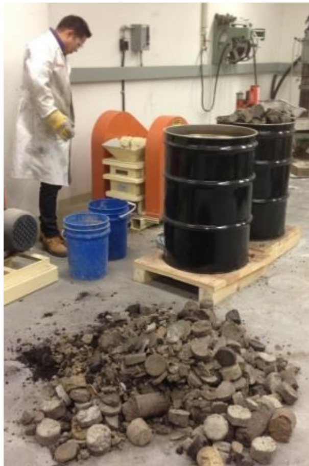
Figure 6-2 Excluding coal layers during crushing in-situ core samples
