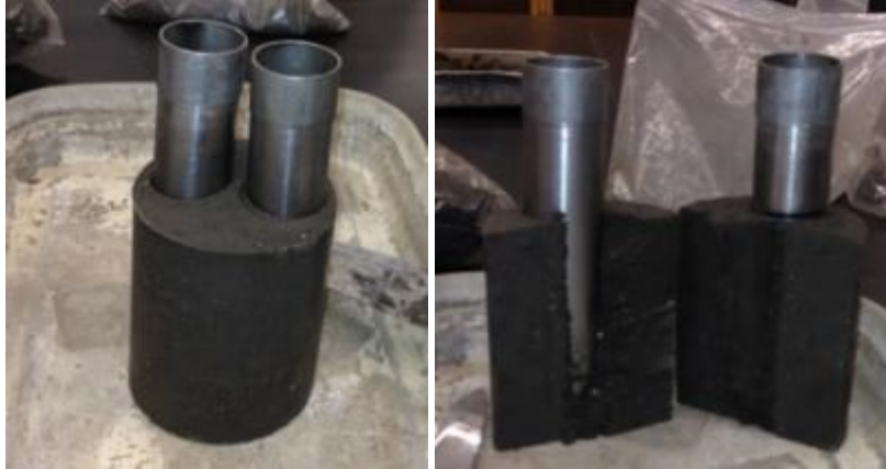
Figure 5-21 Shelby tubes inside the remolded soil samples
