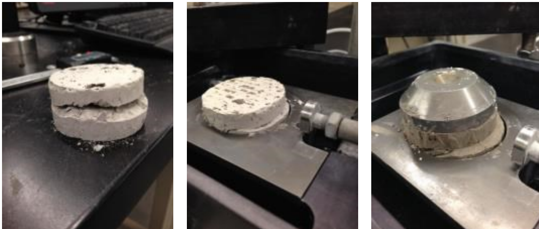
Figure 6-23 Direct shear test on soilcrete cores
