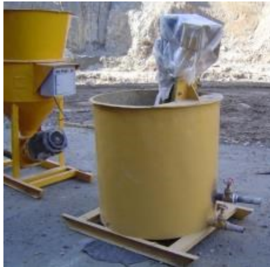
Figure 4-2 Agitator and mixing unit to mix the grout; internal diameter 96cm; depth 90cm
