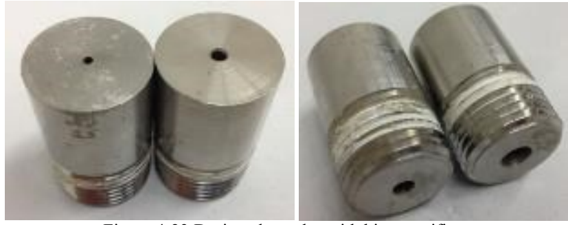
Figure 4-23 Designed nozzles with bigger orifices
