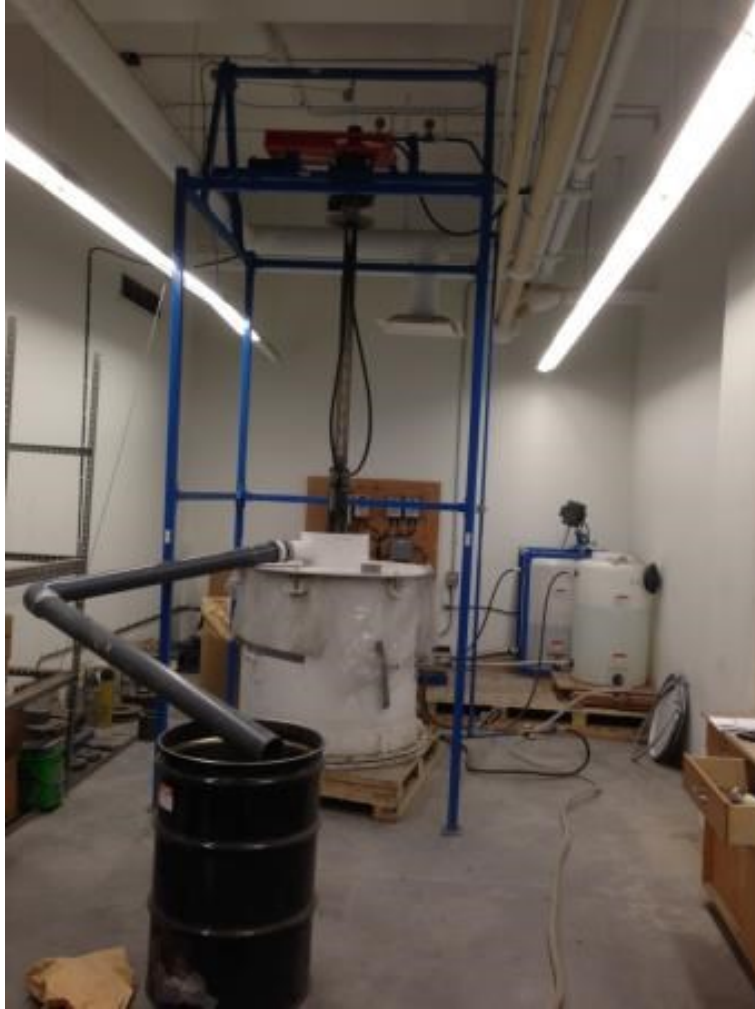
Figure 6-15 Laboratory jet grouting operation
