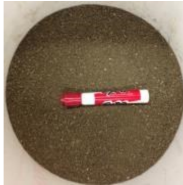
Figure 5-6 Maximum particle size passes sieve No.4 after grinding
