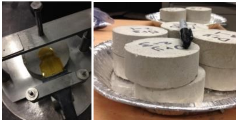
Figure 5-73 Soilcrete samples for thermal properties test
