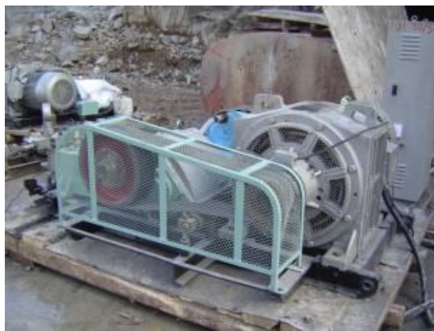
Figure 4-3 Water high pressure pump; maximum pressure: 50MPa and maximum flow rate: 70lit/min
