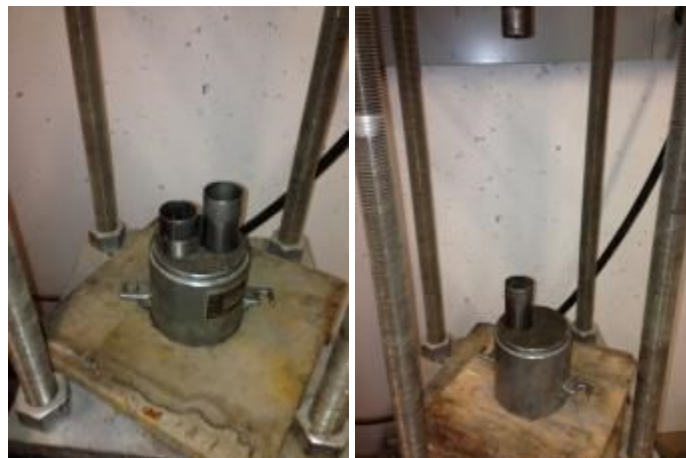
Figure 5-20 Pushing Shelby tubes through remolded soil samples
