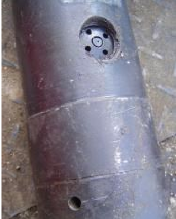
Figure 4-10 Water, air, and grout nozzles in triple fluid monitor
