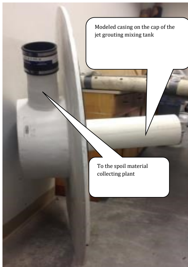
Figure 4-34 Modeling of casing on the cap of the jet grouting mixing tank
