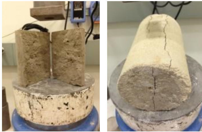
Figure 6-20 STS test on soilcrete cores
