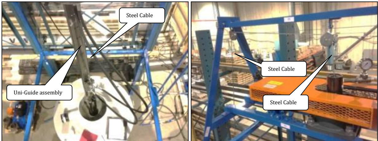
Figure 4-26 Uni-Guide assembly and steel cable of vertical motion
