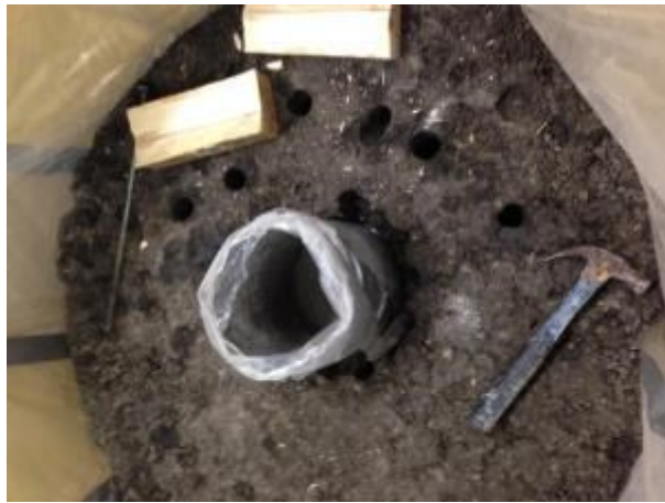
Figure 6-7 Extracting soil samples from reconstructed and compacted soil
