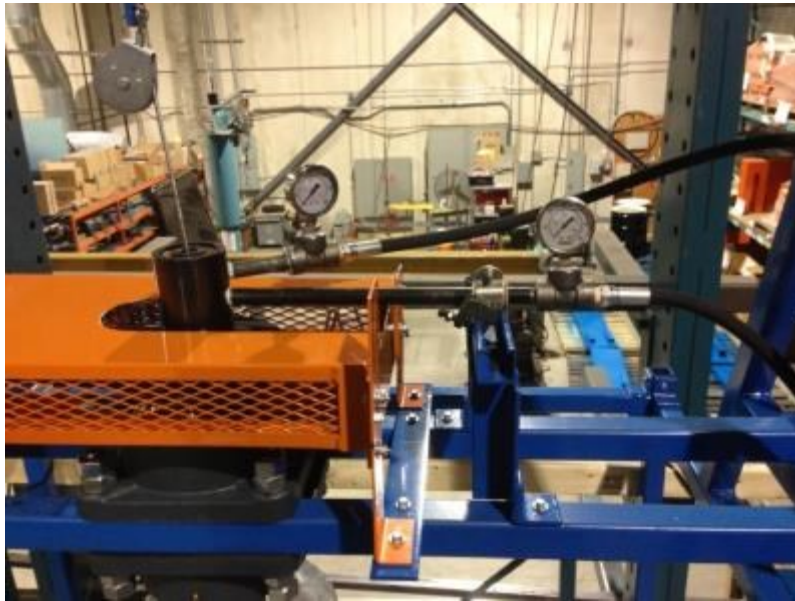
Figure 4-19 Pressure gauges on top of the frame before rotary union
