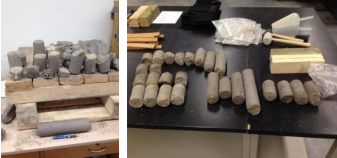
Figure 6-17 Cores extracted from soilcrete body in jet grouting tank
