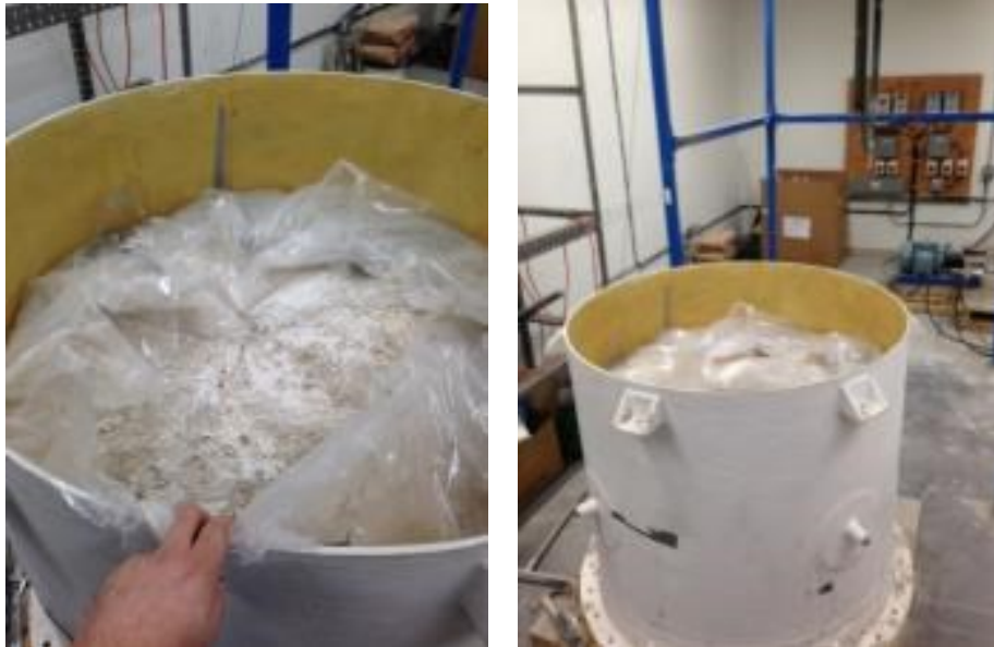
Figure 6-16 Soilcrete mixture in laboratory jet grouting tank
