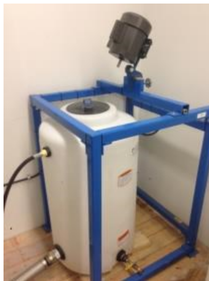
Figure 4-20 Grout mixing plant
