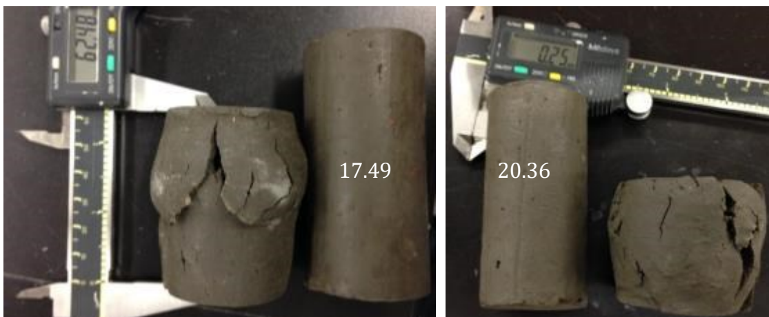
Figure 5-27 Failure of specimens under UCS test for 17.49%, 20.36%
