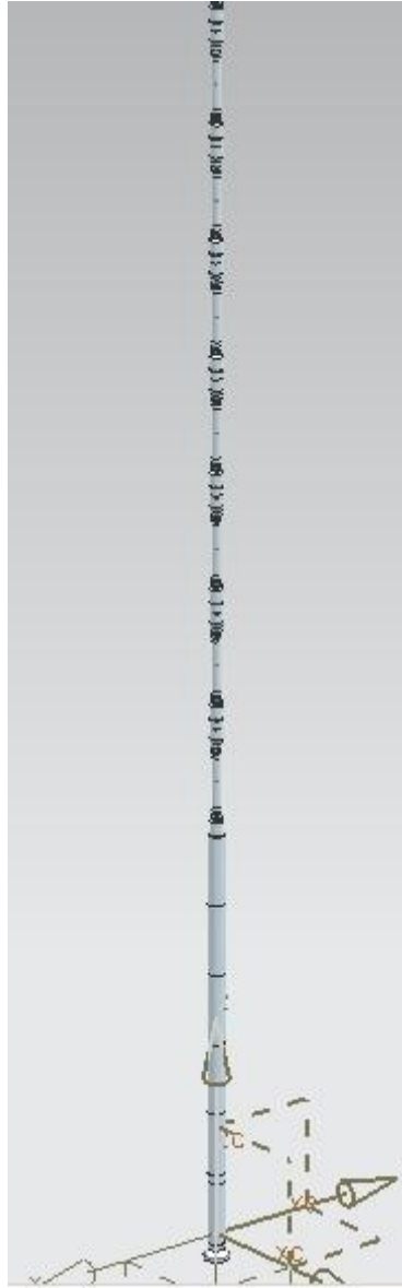
Figure 5-8: Partial assembly of drill string
