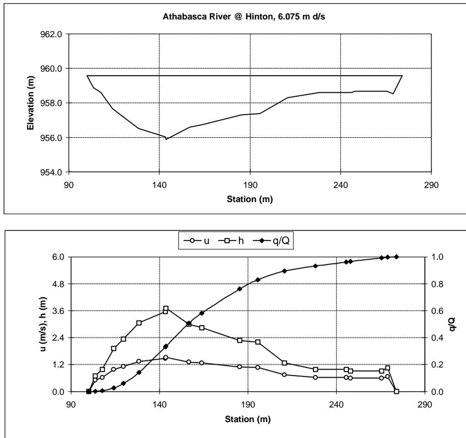
**Figure 4 Example cross section plot.**
