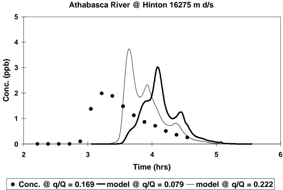
**Figure 10 Athabasca River, c-t curve at 16275 m,  $334 \text{ m}^3/\text{s}$ , slug input.**
