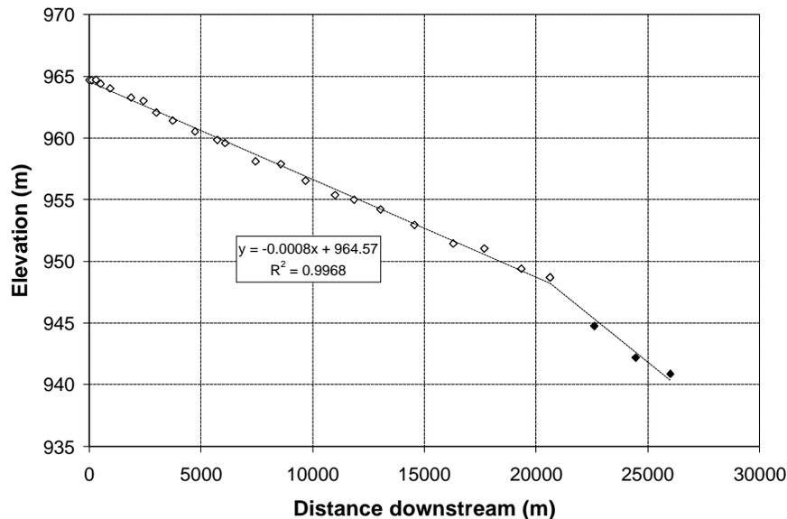
**Figure 5 Water surface elevation versus distance.**
