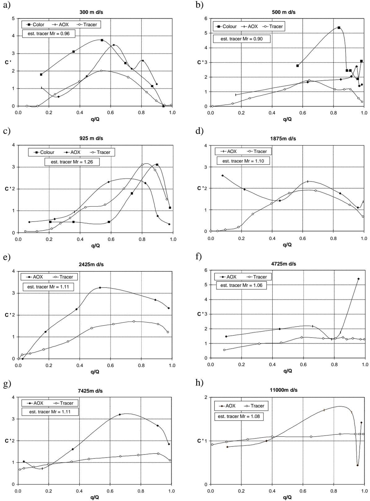
Figure 15 Tracer and water quality parameter dimensionless concentrations.
