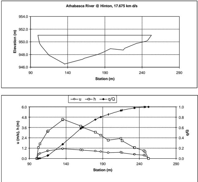
**Figure A21 Cross Section - 17.675 km d/s**
