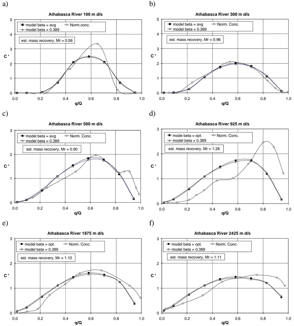
**Figure 7 Normalized dimensionless tracer concentration versus  $q/Q$ .**
