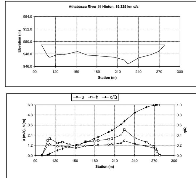
**Figure A22 Cross Section - 19.325 km d/s**
