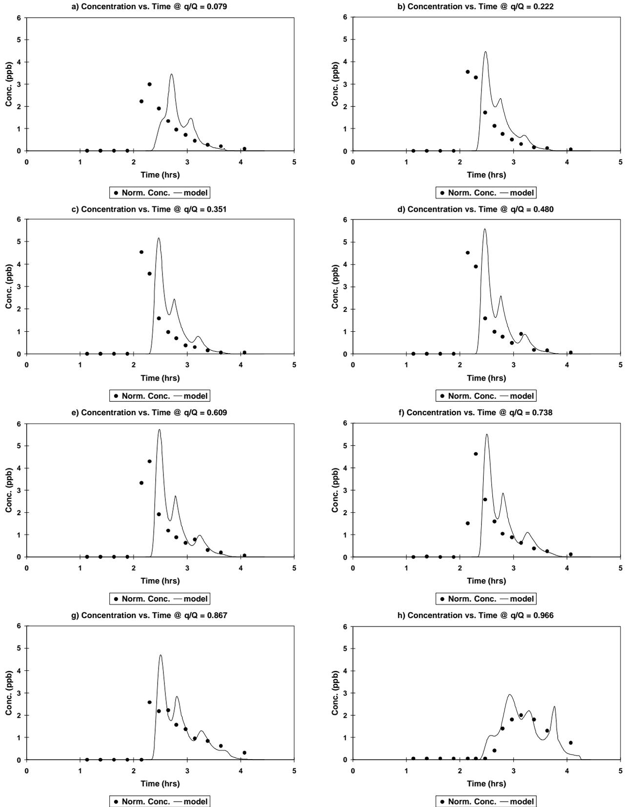
Figure 11 Athabasca River, c-t curves at 11850 m,  $334 \text{ m}^3/\text{s}$ , slug input.
