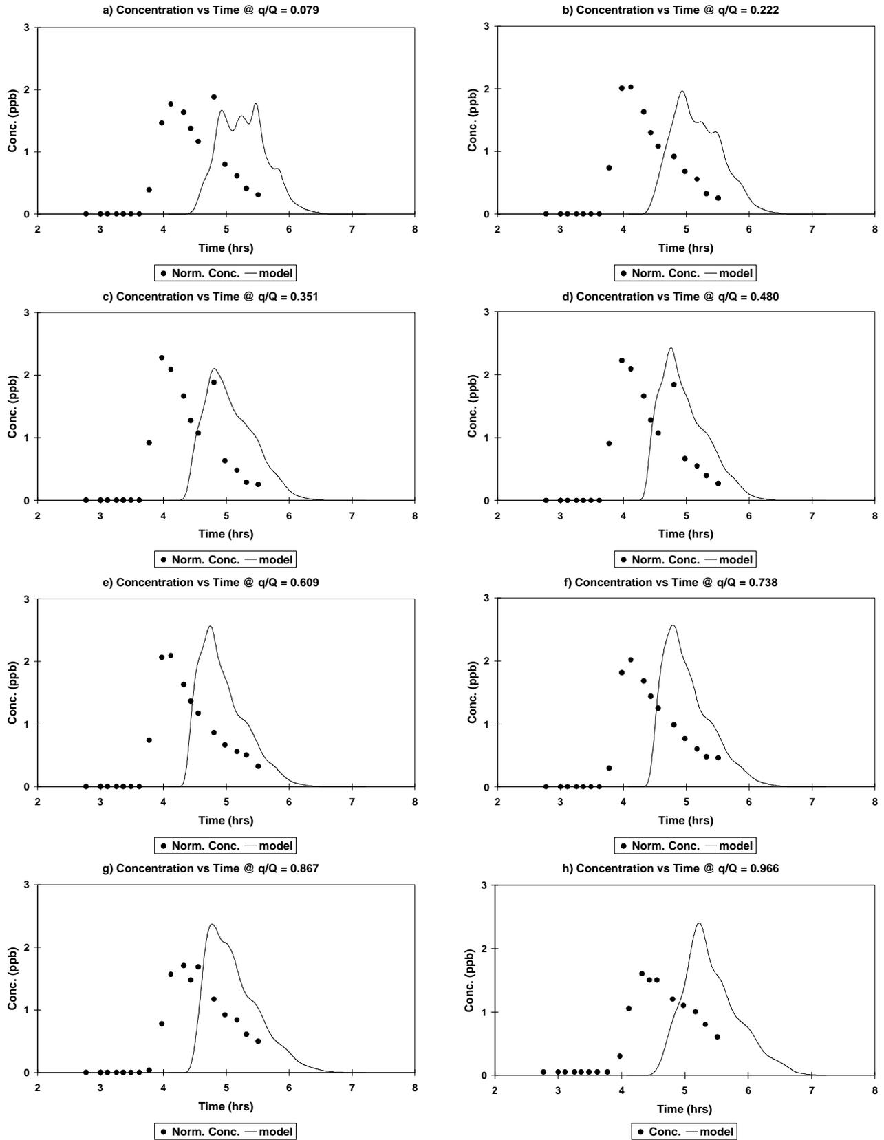
Figure 12 Athabasca River, c-t curves at 20625 m,  $334 \text{ m}^3/\text{s}$ , slug input.
