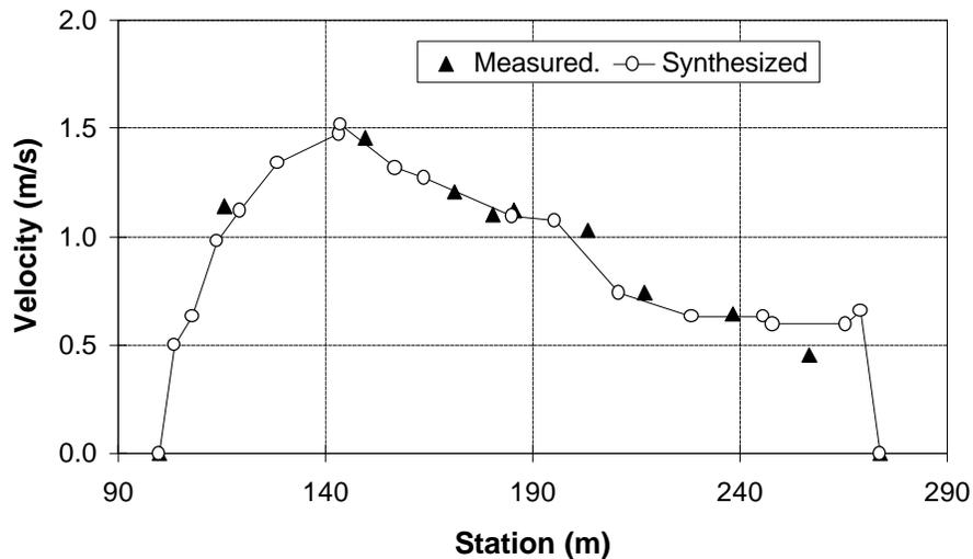
**Figure 6 Measured and synthesized velocity distribution at 6075 m downstream.**
