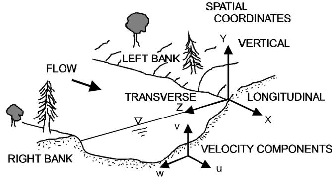
**Figure 1 Coordinate system for mixing analysis.**
