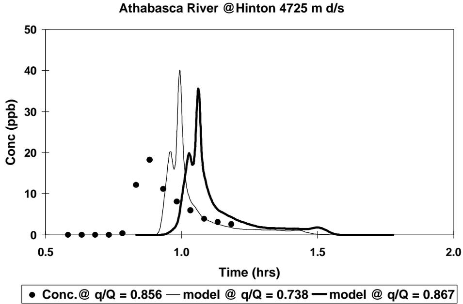
**Figure 9 Athabasca River, c-t curve at 4725 m,  $334 \text{ m}^3/\text{s}$ , slug input.**
