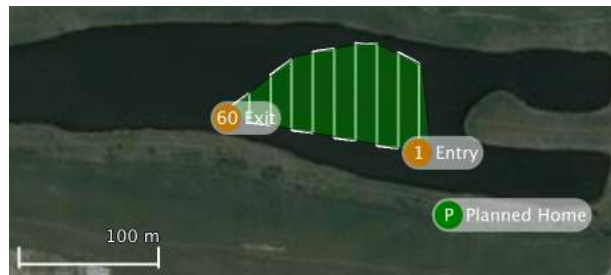
Figure 5. Planned trajectory for surveying part of a natural pond with 15m spacing
