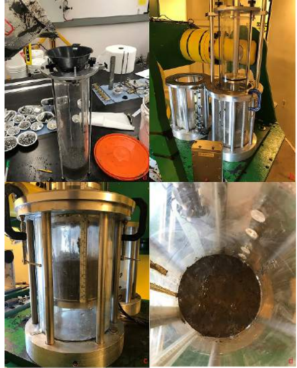
Figure 5. Dispensing Tailings Material to the Consolidation Cell. a) Material is added to the dispenser; b) Dispenser is secured to the consolidation cell; c) Dispenser shown inside consolidation cell; d) Dispensed material in the consolidation cell
