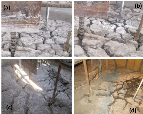
Figure 8. Photographs of the surface of cake in Column 1 showing atmospheric drying, taken on: (a) April 2015; (b) July 2015; (c) September 2015; and (d) December 2015)
