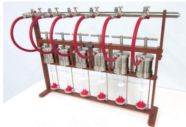
Figure 1. Specific Resistance to Filtration (SRF) setup (Figure adopted from OFITE website)
