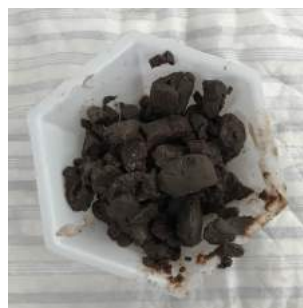
Figure 4b. Solids recovered from filter backwash after decanting only. The solids are suitable for trucking without further processing
