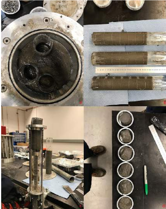
Figure 2. Push Tube Sampling Technique. a) Push tubes are inserted into sample; b) Push tubes are removed from sample; c) Push tubes samples are extruded in equal heights; d) Six samples obtained from push tubes prior to oven-drying
