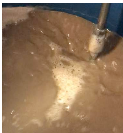
Figure 3b. Treatment feed water of 50/50 EBD/SAC Regen with chemicals. Note high solids content
