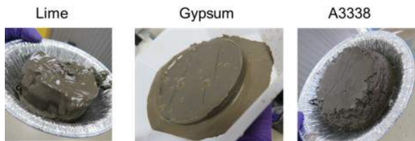
Figure 12. Photos of SRF cakes obtained by 300 g of treated FFT with 60 minutes test and unmodified setup
