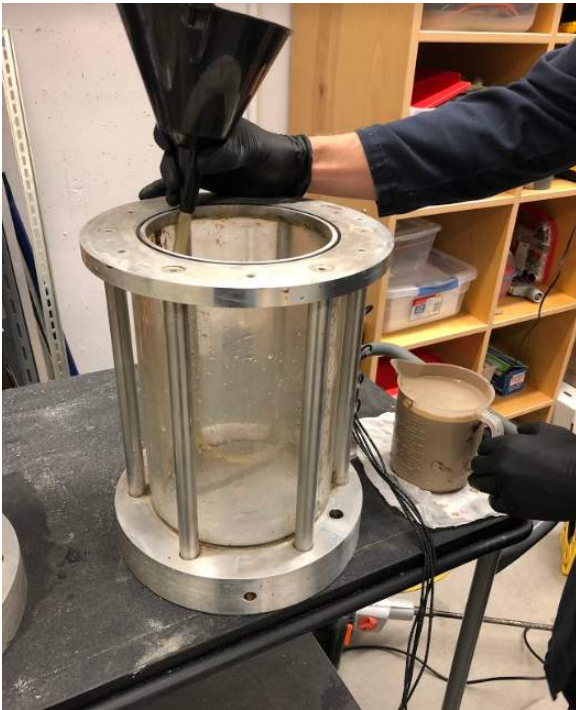
Figure 4. Funneling Kaolinite Slurry into Consolidation Cell
