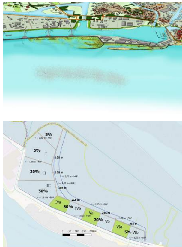
Figure 5. Infographic representing the development of salt marshes in front of the Delzijl harbor entrance channel (top), and the design of the Marconi salt marsh with the specific subdivision in different compartments with different fines content to be mixed in sand (5 – 20 – 50%), green represents sections where vegetation will be planted (bottom)
