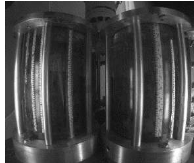
Figure 5. Tracking the tailings settlement in-flight
