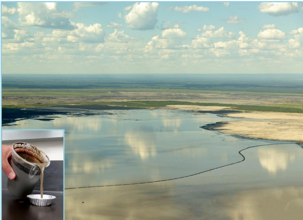
Figure 2-1 Fluid fine tailings have a muddy water consistency
