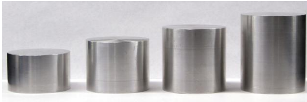
Figure 6-A1 Set of Aluminum 6061-T6 used to calibrate P- and S- travel times shown at increasing length.
