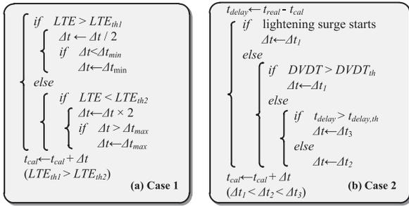
Fig. 7. Pseudocode for the time-step control module. (a) Diode full-bridge circuit. (b) Power transmission system.
