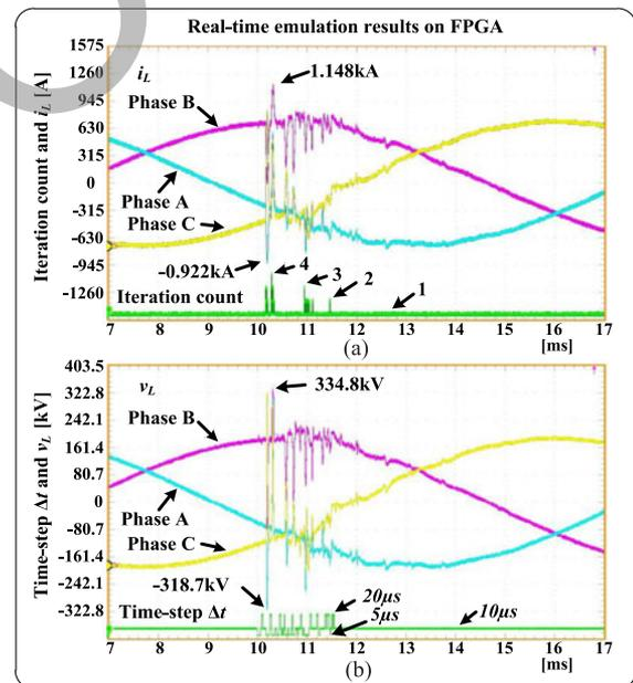
**Fig. 10.** Real-time emulation results on the FPGA captured by an oscilloscope for the power transmission system case study. (a) Load current  $i_L$  and iteration count. (b) Load voltage  $v_L$  and time step  $\Delta t$ .
