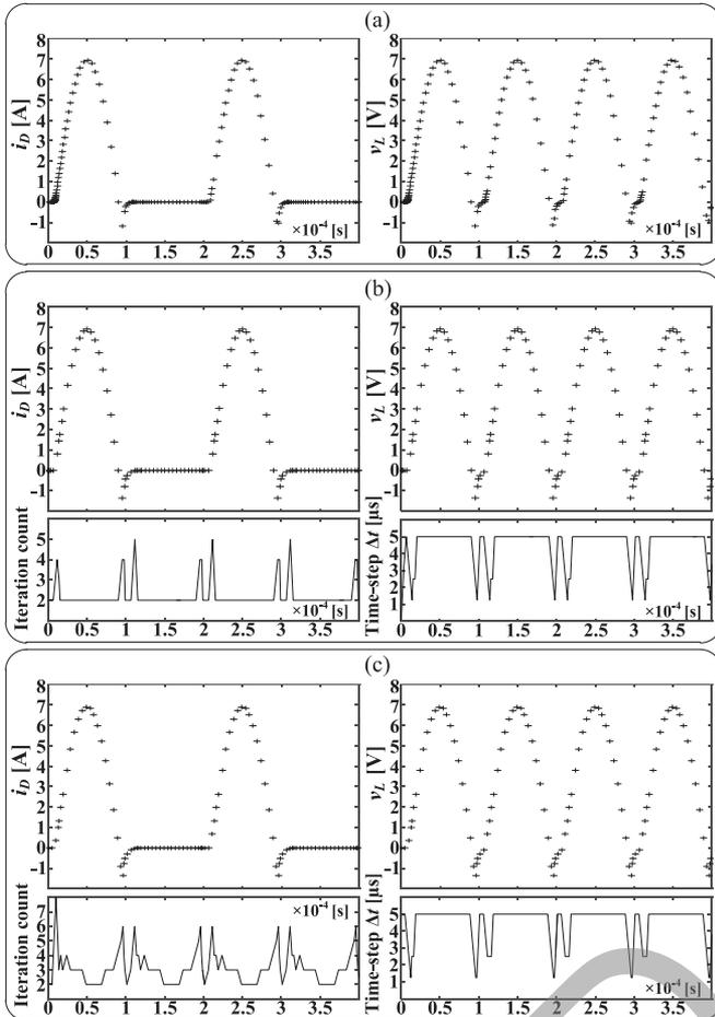
Fig. 2. Offline results of diode current  $i_D$  for  $D_1$ , load voltage  $v_L$ , iteration count, and time step  $\Delta t$ . (a) Saber. (b) LTE scheme based on the N-R method. (c) Iteration count scheme based on the N-R method.
