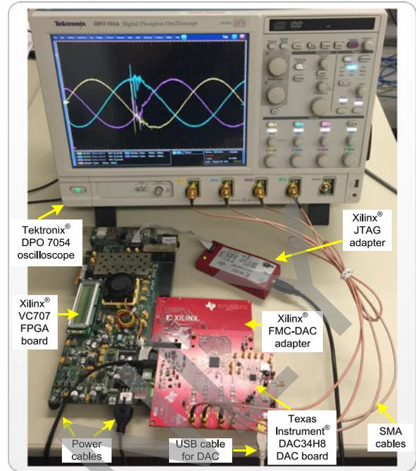
Fig. 8. Hardware setup for the FPGA-based real-time emulation.
