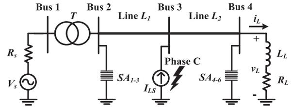
Fig. 3. Single-line diagram for the power transmission system case study.
