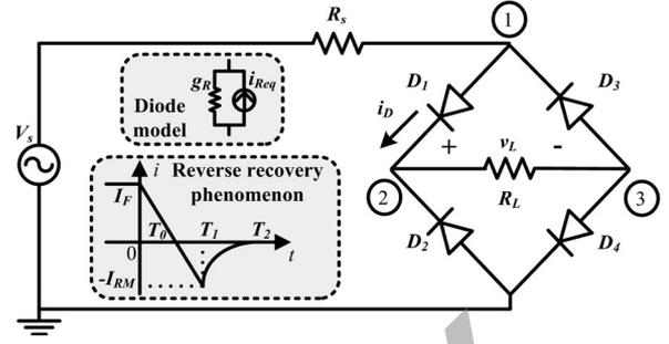
Fig. 1. Circuit topology, the diode model, and the reverse recovery phenomenon for the diode full-bridge circuit case study.
