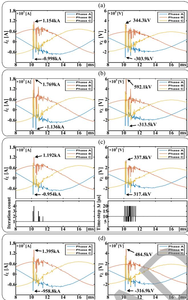
Fig. 4. Offline results of load current  $i_L$ , load voltage  $v_L$ , iteration count, and time step  $\Delta t$ . (a) PSCAD/EMTDC with a fixed time step  $5 \mu\text{s}$ . (b) PSCAD/EMTDC with a fixed time step  $10 \mu\text{s}$ . (c) DVDT scheme based on the PNR method. (d) DVDT scheme based on the PL method.
