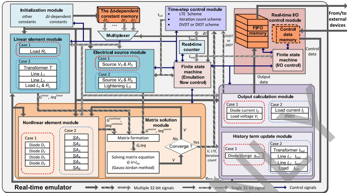
Fig. 5. Hardware implementation and data flow of the real-time emulator for the case studies.
