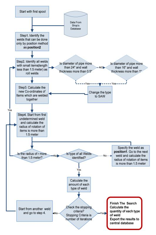
Figure 2.9 Heuristic search algorithm used for determining types of welds
