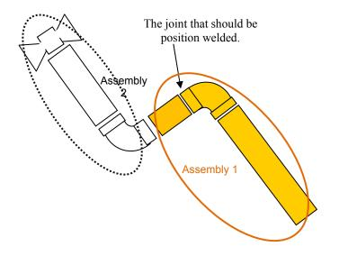
Figure 2.2 Assembly parts of a spool
