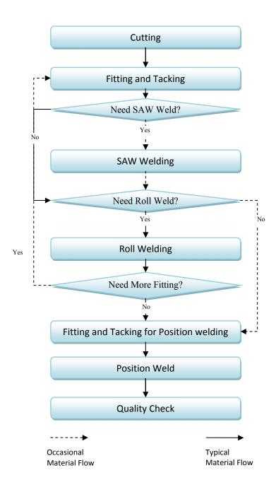
Figure 2.4 Flowchart of pipe spool fabrication process
