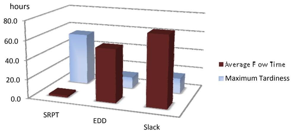
Figure 3.5 Simulation results of applying three simple dispatching rules on a spool fabrication shop (maximum tardiness vs. average flow time)
