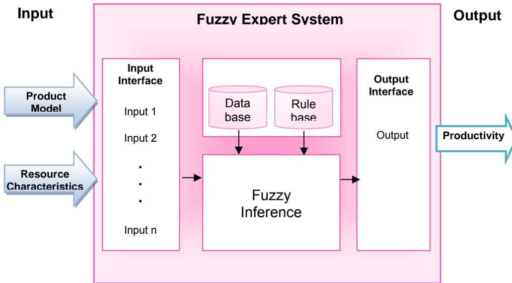
Figure 2.14 The structure of fuzzy expert system
