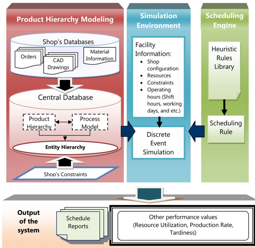
Figure 2.6 Architecture of proposed framework for industrial fabrication scheduling
