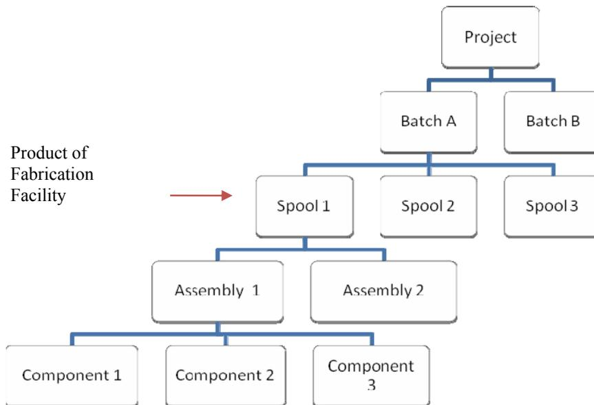
Figure 2.7 Typical work breakdown structure for spool fabrication
