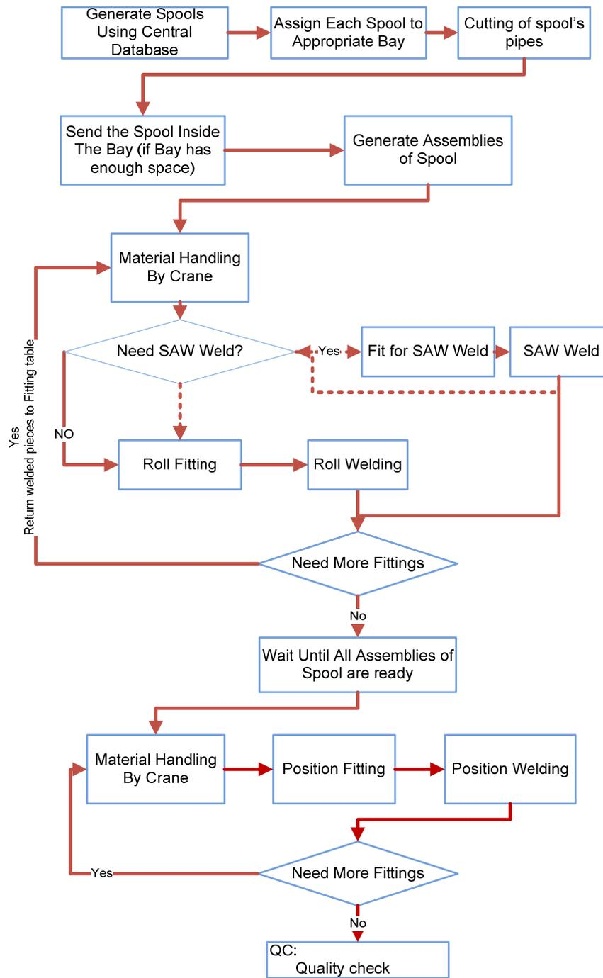
Figure 4.2 Structure of simulation model for case study
