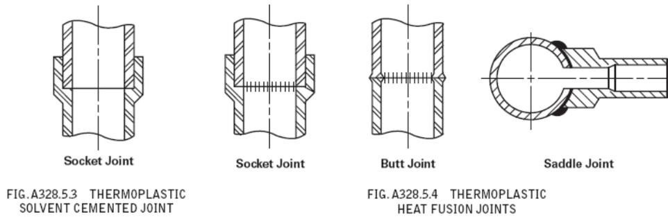
Figure A1 Socket weld and butt weld
