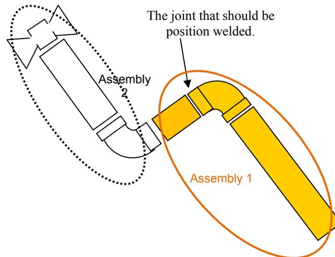
Figure 2.2 Assembly parts of a spool
