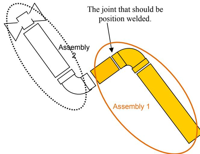
Figure 2.2 Assembly parts of a spool
