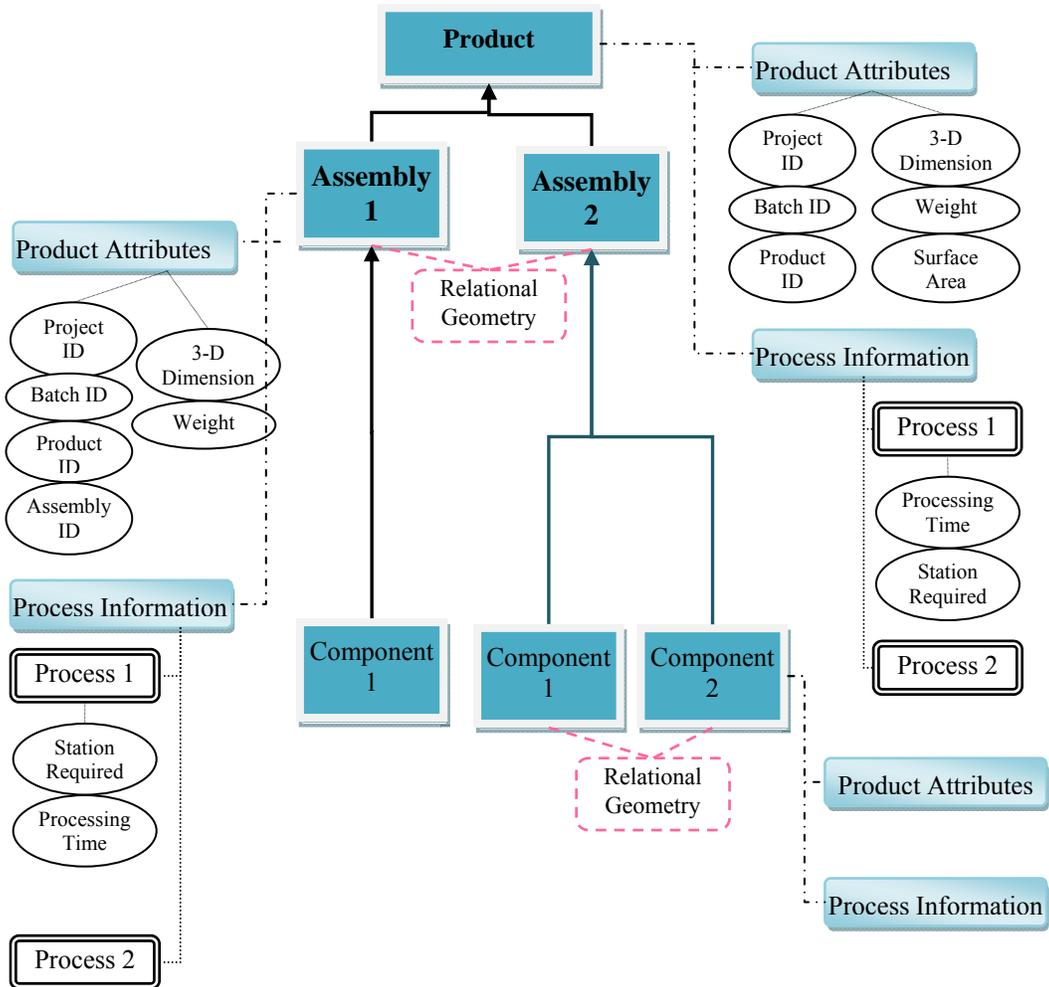
Figure 2.12 Process model for spool in relation to spool's product model
