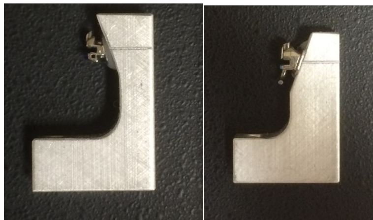
Figure 3- 2: Brackets bonded to aluminum dowels
