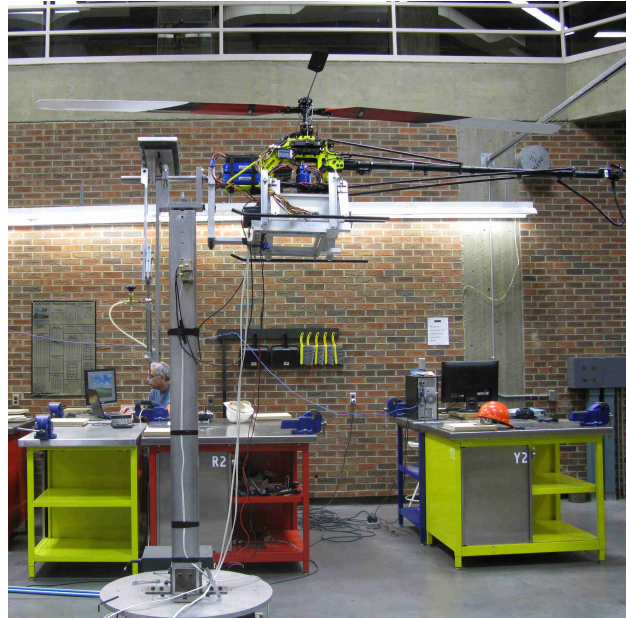
Figure 7.6: HIL testbed setup for the roll control in hover.
