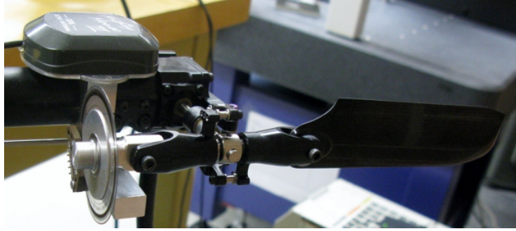
Figure 4.5: The measurement setup for the tail rotor mechanism.
