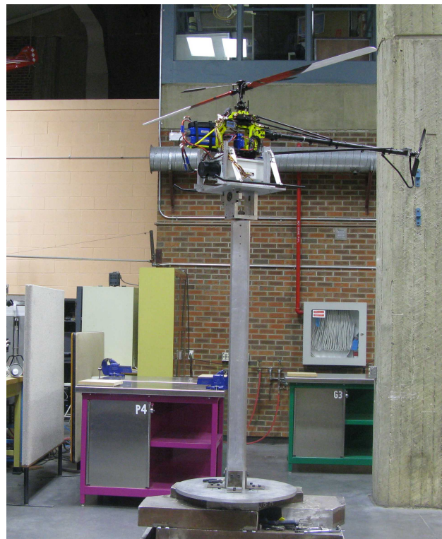
Figure 7.7: HIL testbed setup for the yaw control.
